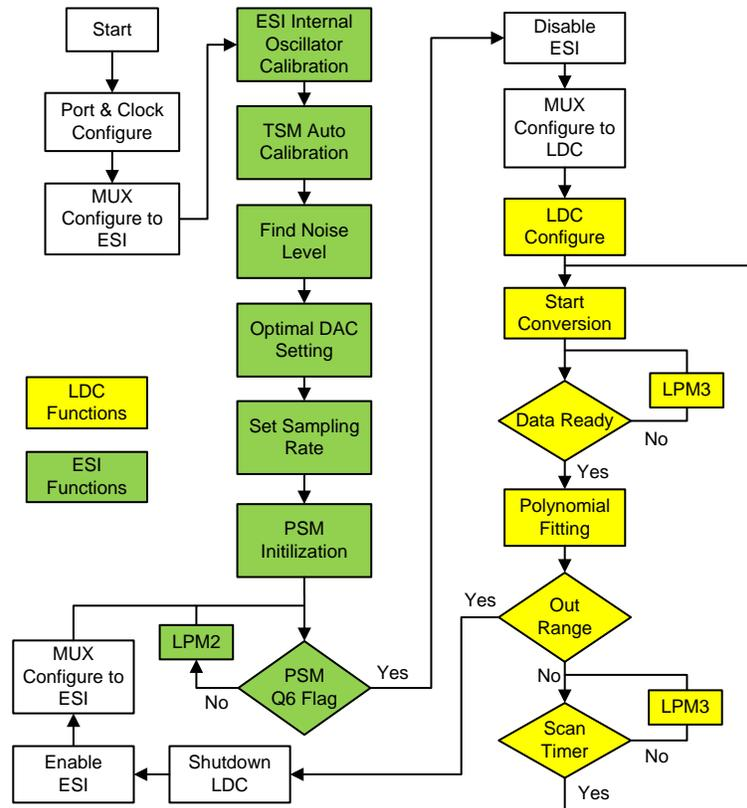
Figure 13. Flowchart of the Firmware
