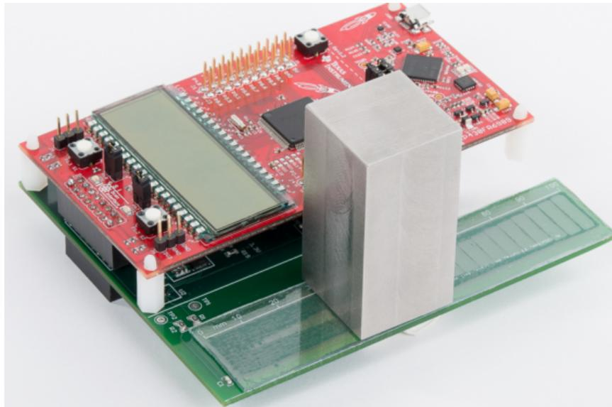
**Figure 12. Inductive Linear Position Sensing Reference Design and Metal Target**
