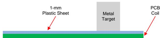
**Figure 9. Moving Target With 1 mm Gap (Side View)**
