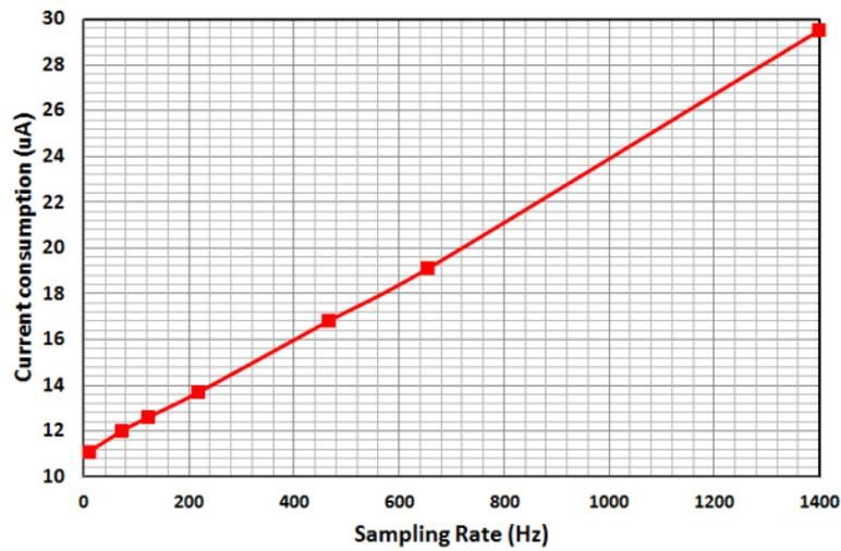
Figure 24. System Power Consumption for ESI Mode
