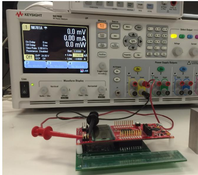
Figure 19. DC Power Analyzer Power Consumption Test Configuration
