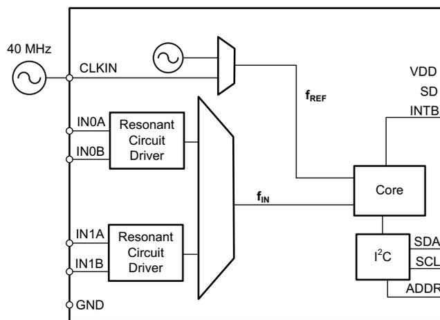
Figure 2. LDC1612 Block Diagram
