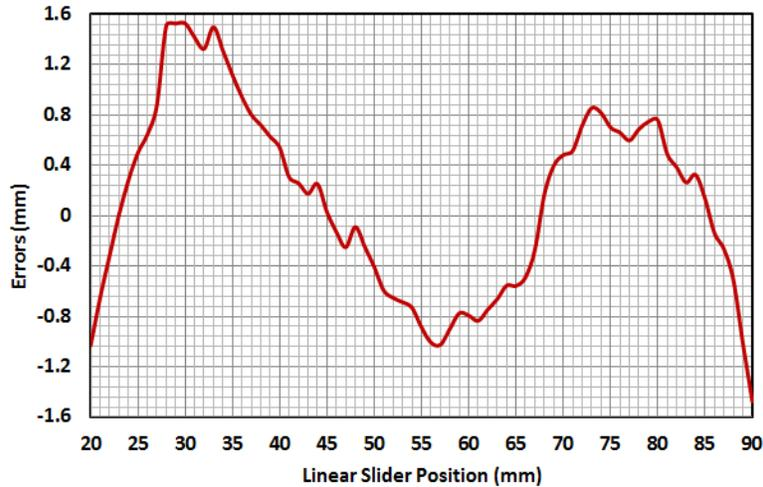
Figure 17. Polynomial Fitting Errors
