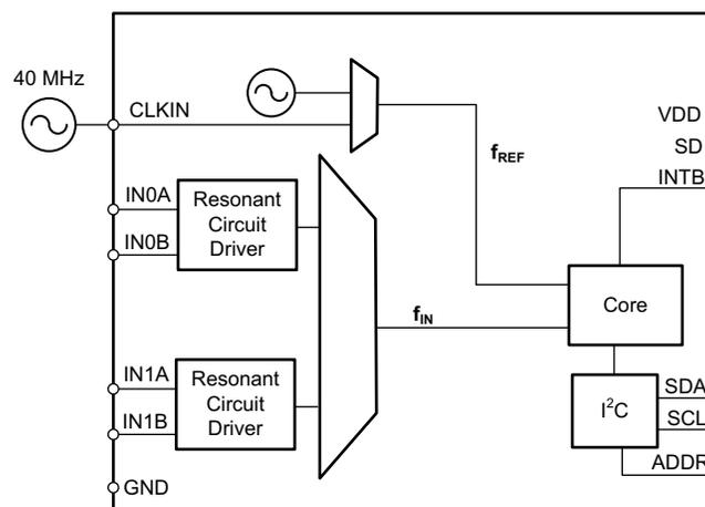
**Figure 5. Functional Block Diagram of the LDC1612**
