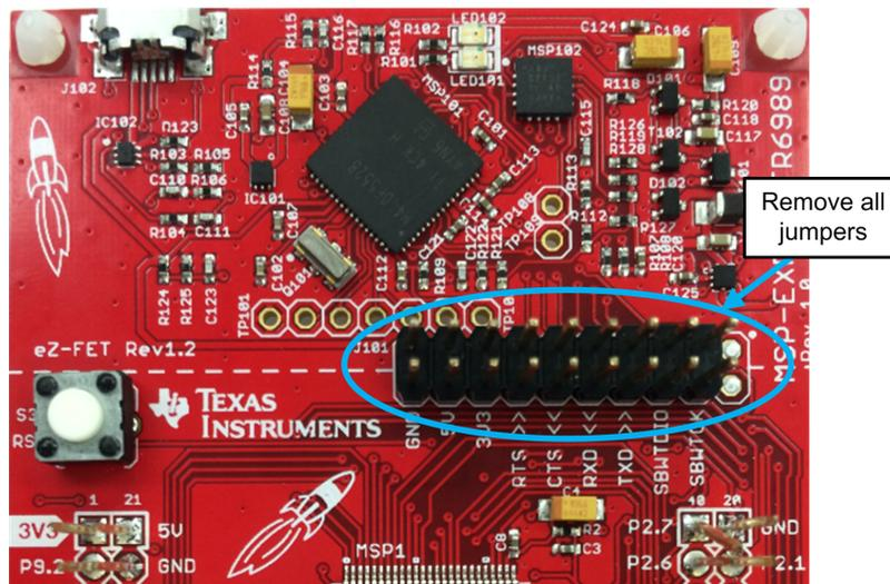
Figure 18. External Power Supply Jumper Configuration
