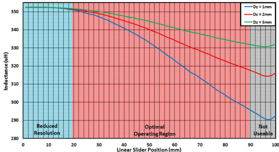
**Figure 23. Sensor Inductance Versus Linear Position**
