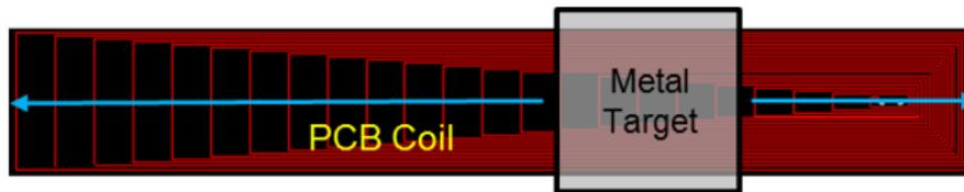
Figure 6. Lateral Movement of Rectangular Target on PCB Coil
