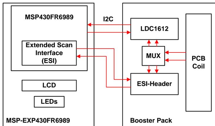
Figure 3. System Block Diagram
