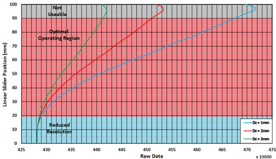
Figure 21. Linear Position Versus LDC1612 Raw Data
