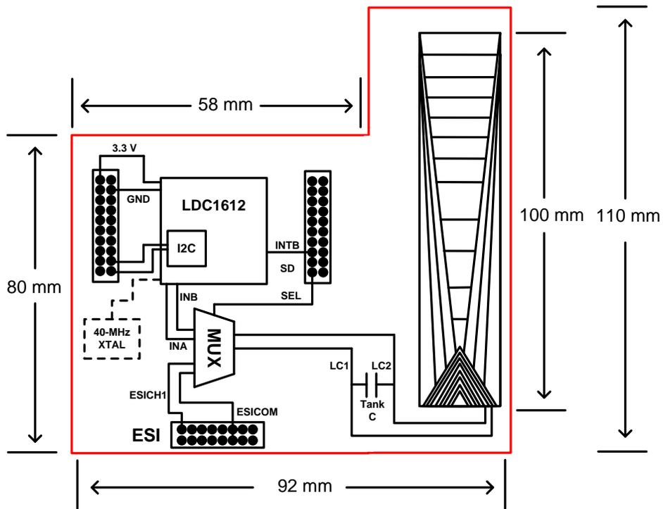
**Figure 4. BoosterPack Diagram**
