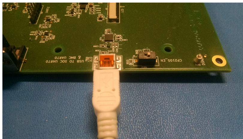
Figure 14. General-Purpose EVM UART to USB Port Connection for Serial Output
