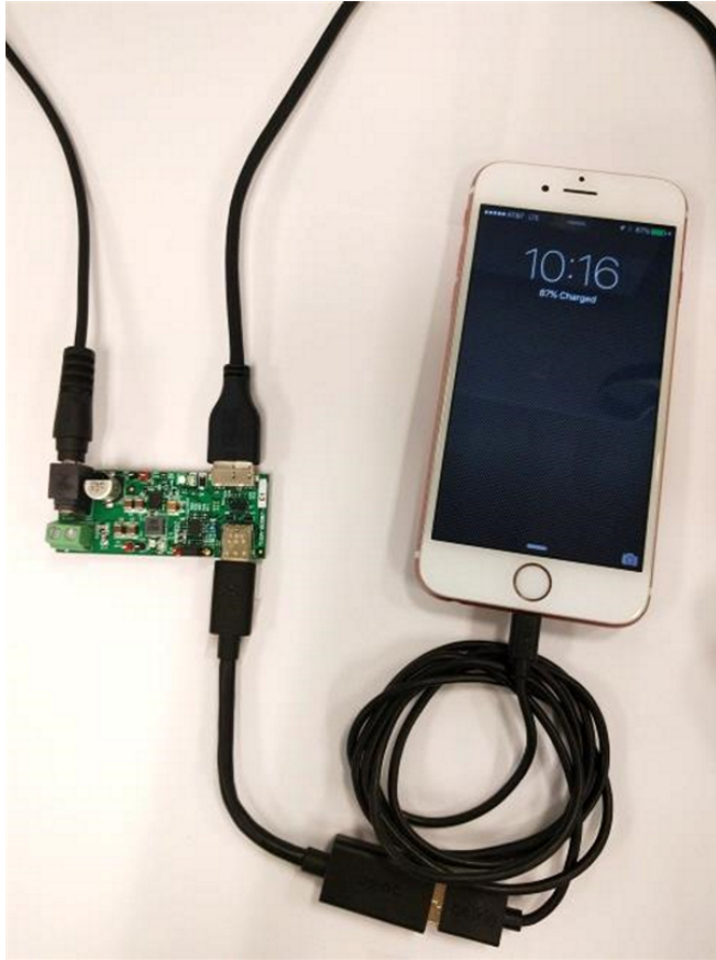
Figure 32. Type-A Needs Host Connection for CDP Mode
