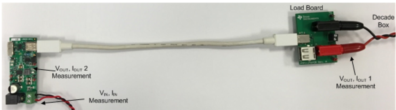
Figure 44. Efficiency Measurement Setup
