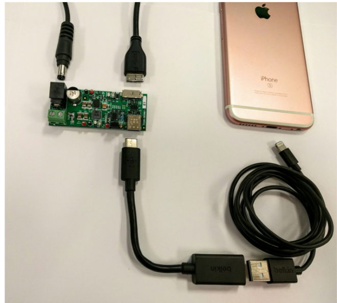
Figure 31. Setup: Type-C to Legacy Type-A Connection
