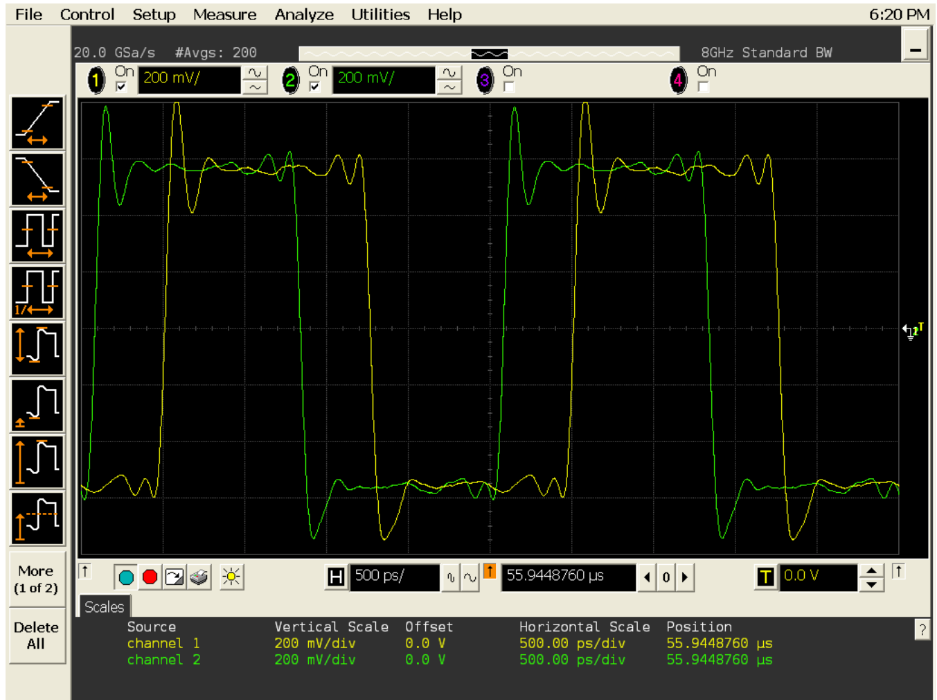
Figure 6. Non-Timing Critical Example Before SYNC Pulse
