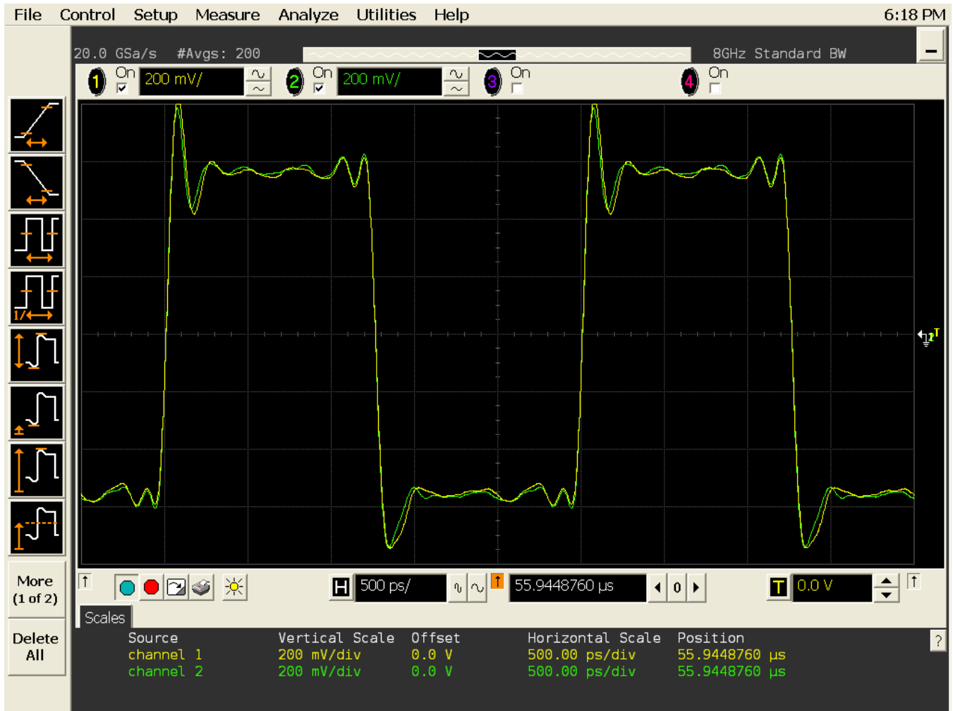
Figure 7. Non-Critical SYNC Example After SYNC Pulse
