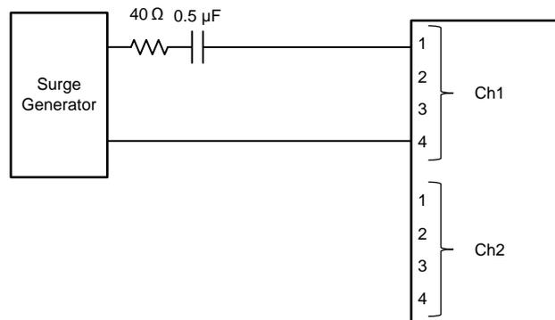
**Figure 6. Surge Test Wiring Diagram**
