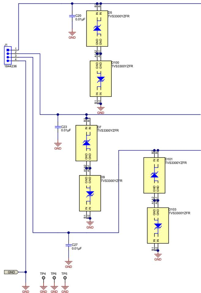
Figure 5. Input Protection Schematic With TVS3300
