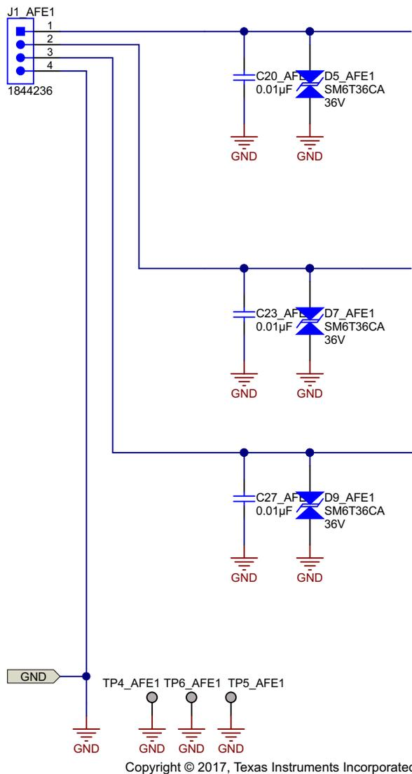
Figure 4. Input Protection Schematic
