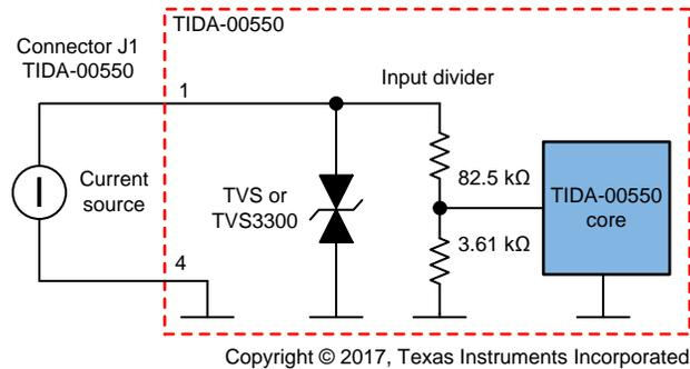
**Figure 1. Block Diagram (One Channel)**
