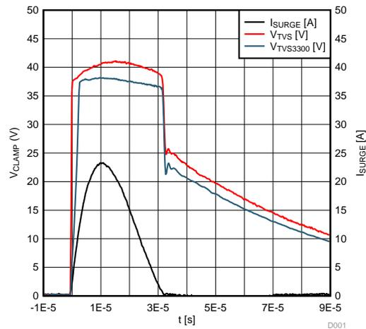
**Figure 7. Clamping Voltage Over Surge Current**
