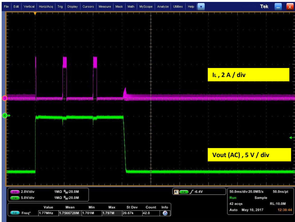
Figure 24: Short circuit response and recovery
