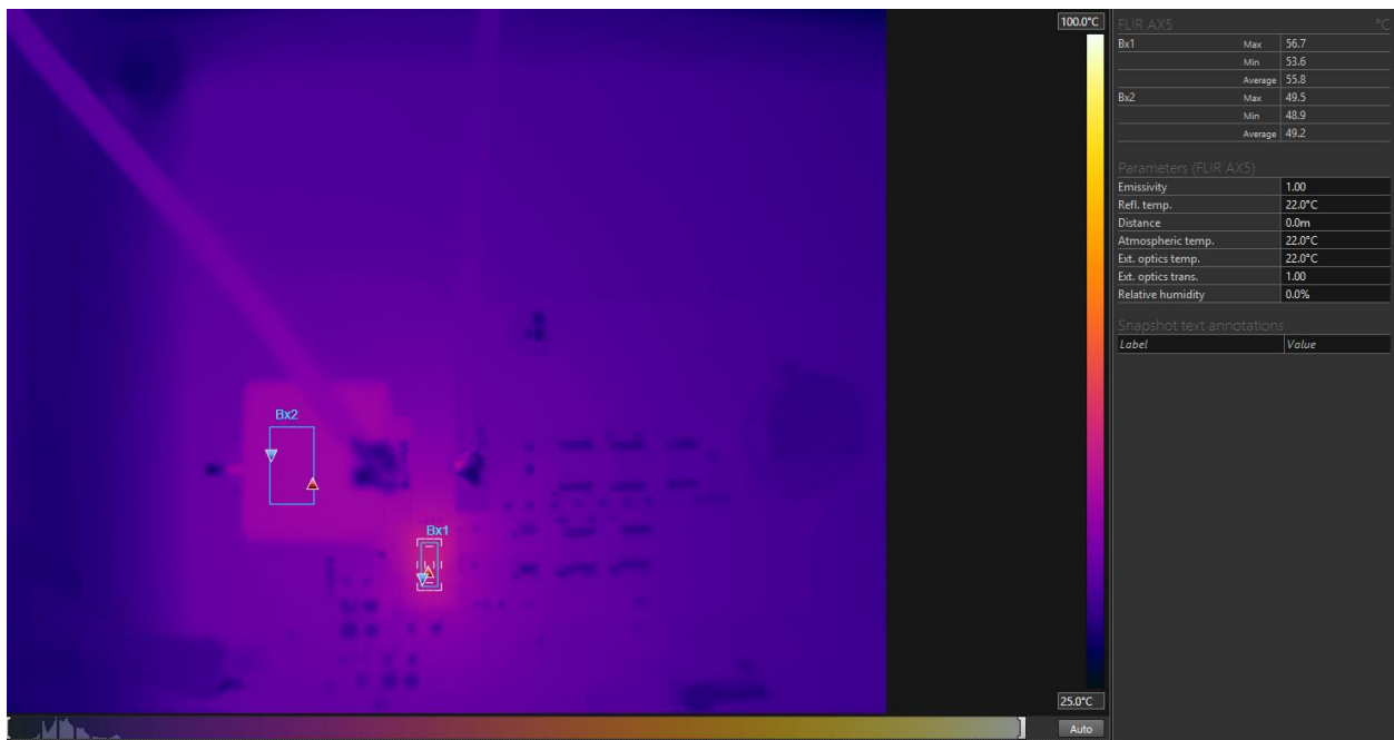
Figure 12: IR thermal image taken at steady state with 24 VIN, -5 Vout and 3 A load (no airflow)
