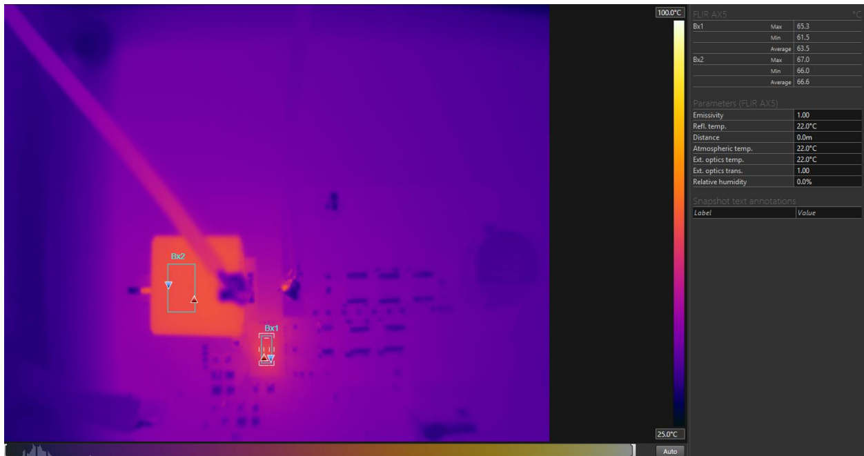
Figure 10: IR thermal image taken at steady state with 24 VIN , -15 Vout and 2 A load (no airflow)
