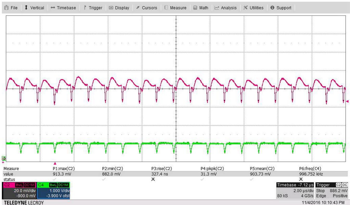
Figure 13. 65-A to 140-A Transient, 1-MHz Load Frequency
