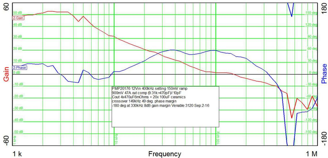
Figure 7. Bode Plot: 50-A Load,  $V_{IN} = 12$  V
