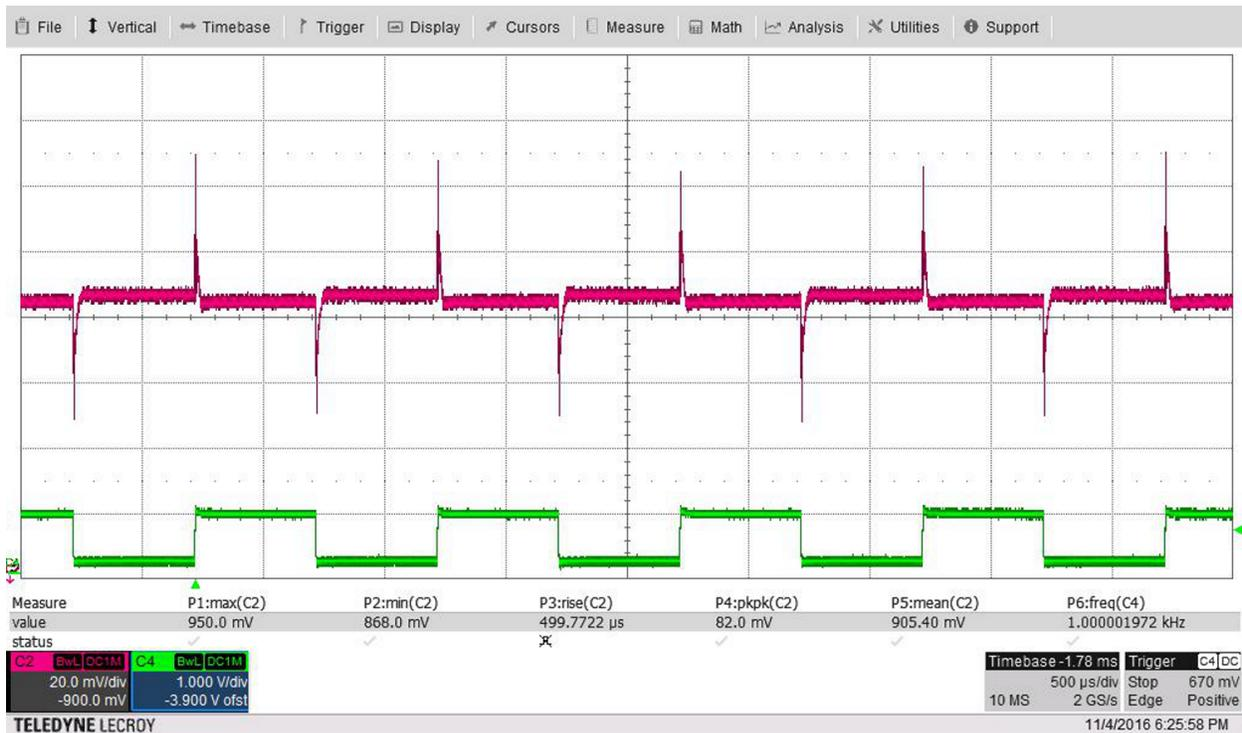
Figure 10. 4-A to 79-A Transient, 1-kHz Load Frequency
