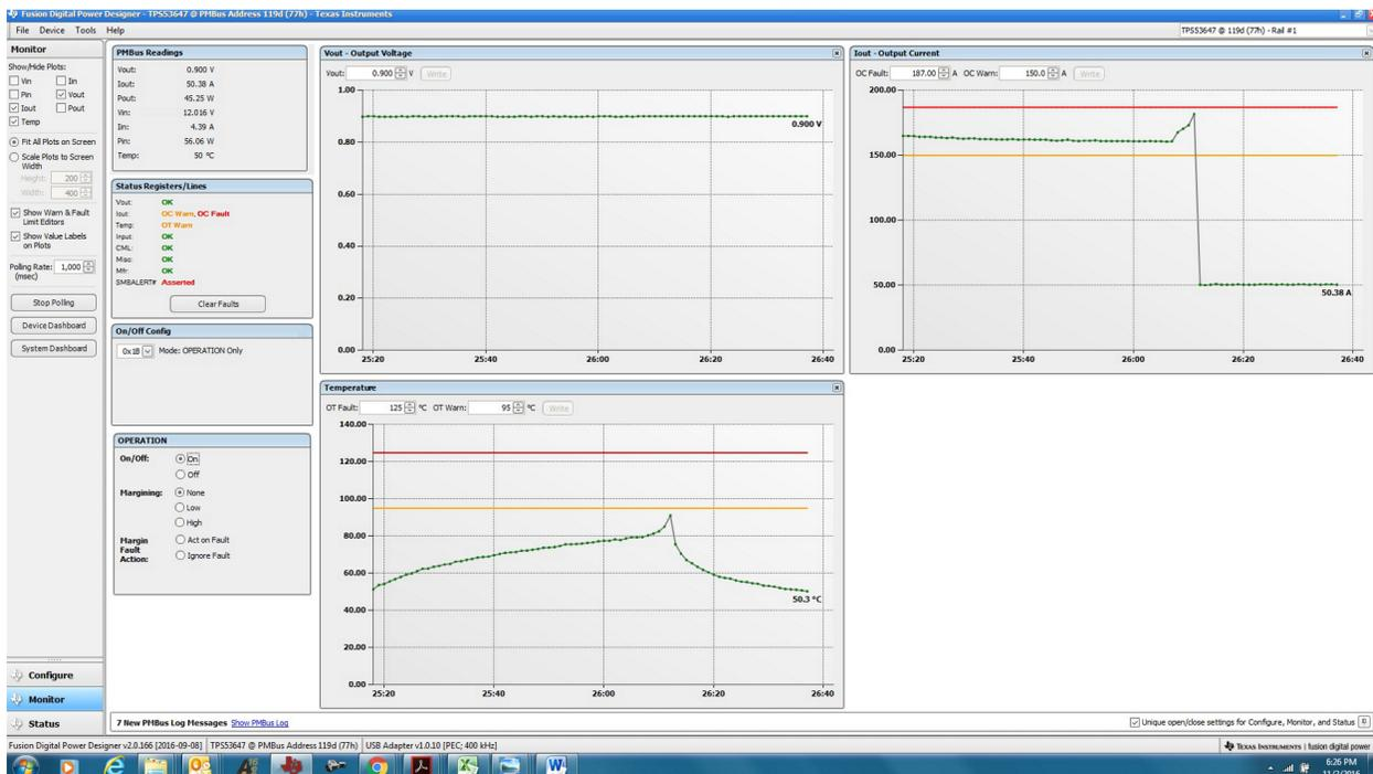
Figure 20. Single Overcurrent Shutdown as Seen in Fusion GUI
