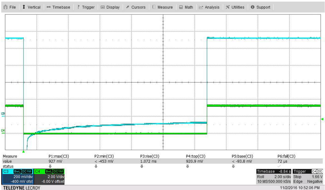
Figure 21. Overtemperature Shutdown With Recovery
