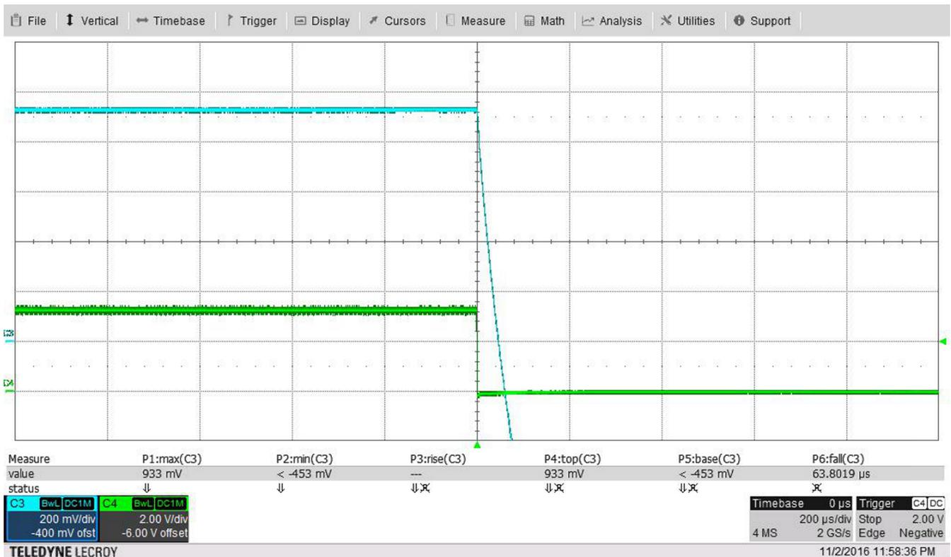
Figure 18. Single Overcurrent Shutdown
