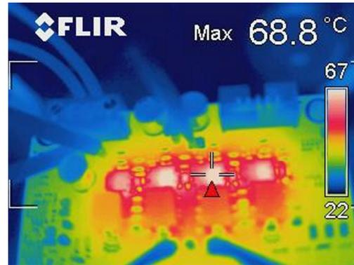
Figure 9. 140-A Load Thermal Performance, ≈350 LFM
