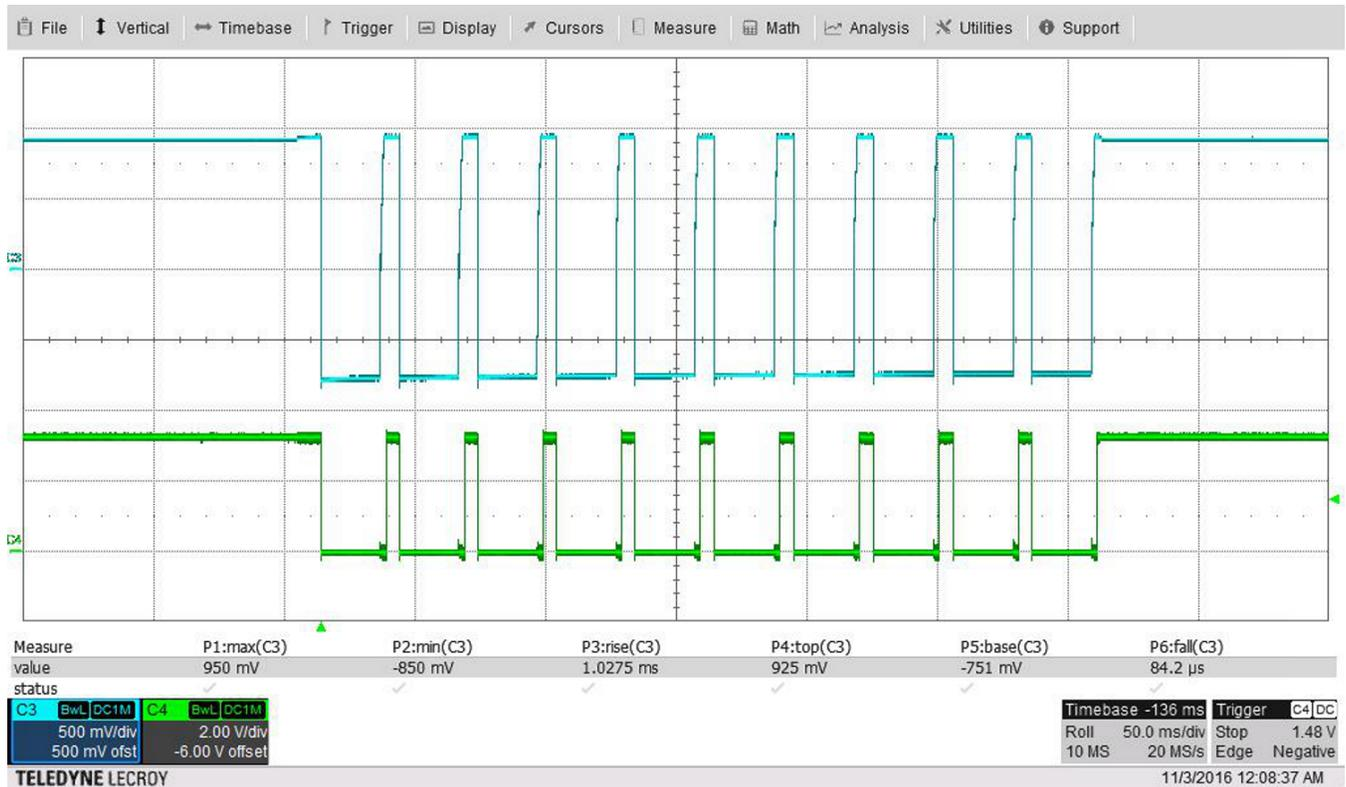
Figure 19. Overcurrent Shutdown With Hiccup Mode
