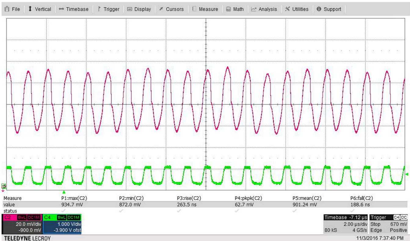
Figure 11. 4-A to 79-A Transient, 1-MHz Load Frequency
