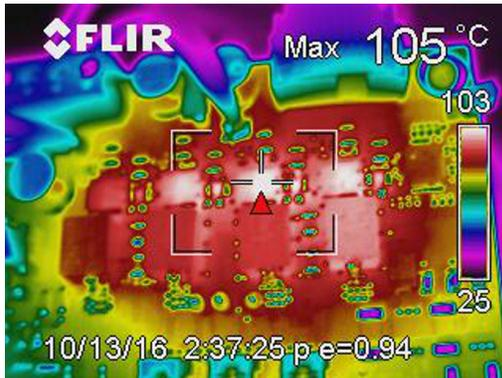
Figure 8. 100-A Load Thermal Performance, No Airflow
