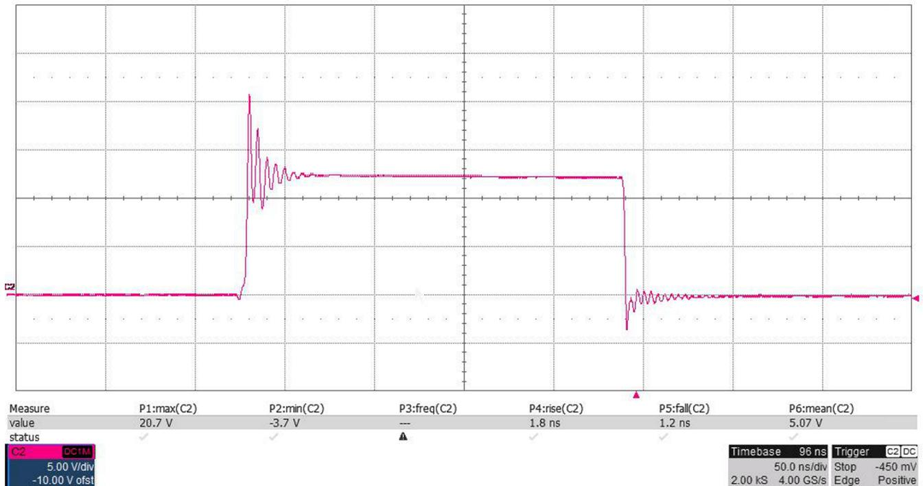
Figure 5. Phase Node Ringing With 40-A Load
