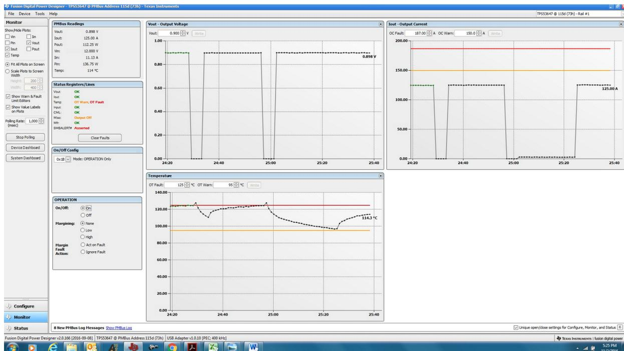
Figure 22. Overtemperature Shutdown and Recovery as Seen in Fusion GUI
