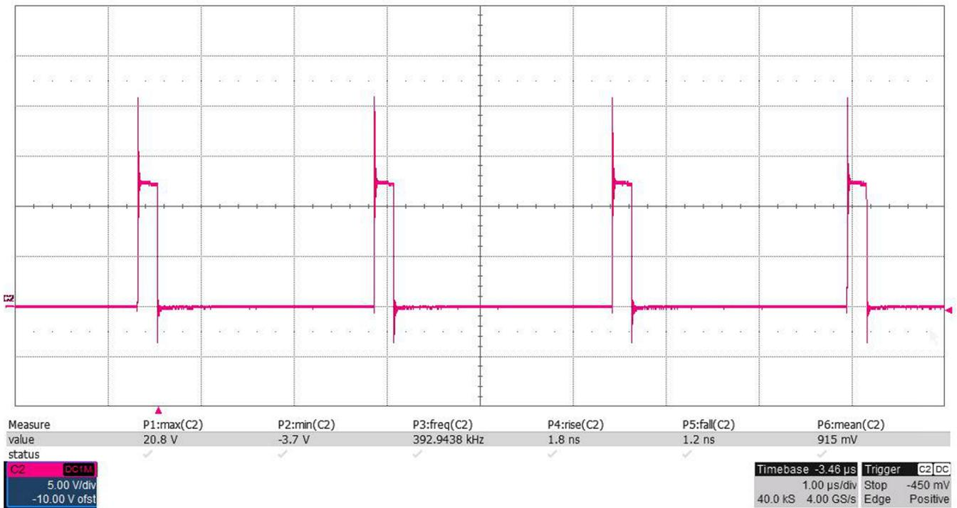
Figure 6. Phase Node Pulses
