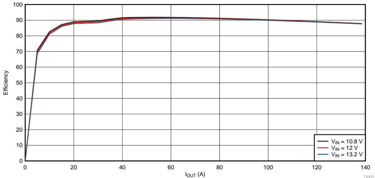
Figure 3. PMP20176 Efficiency Curves:  $V_{OUT} = 0.9\text{ V}$ , 400 kHz
