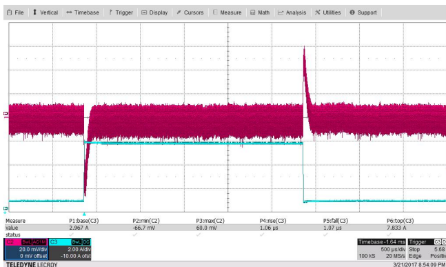
Figure 23. Buck 5-V Output With Load-Step From 3 A to 8 A With Input at 36 V
