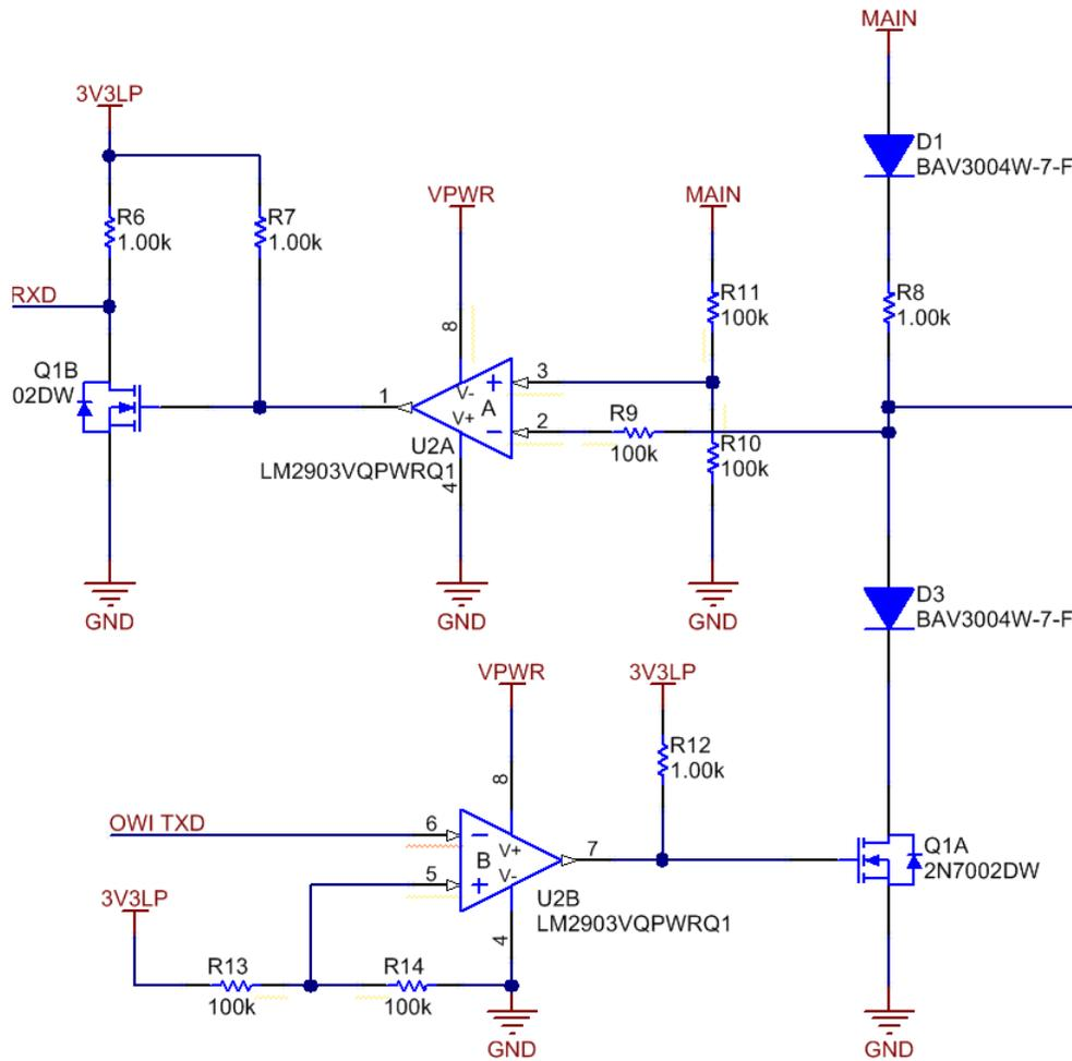
Figure 10. TCI Level Translator Schematic
