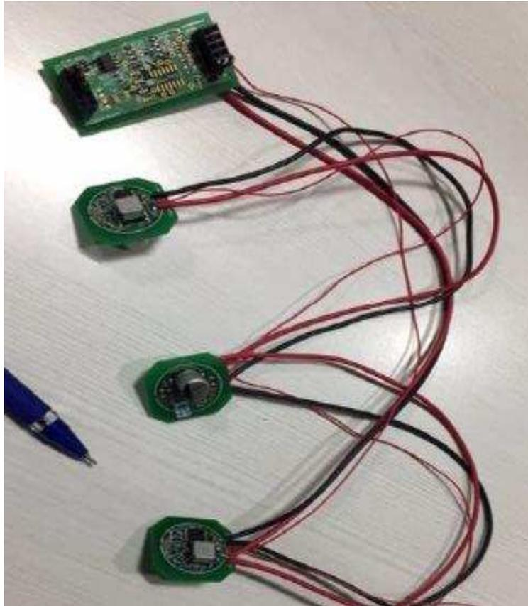
**Figure 14. TIDA-01597 System Hardware - Three Sensor Transducer Boards and an OWI Transceiver**
