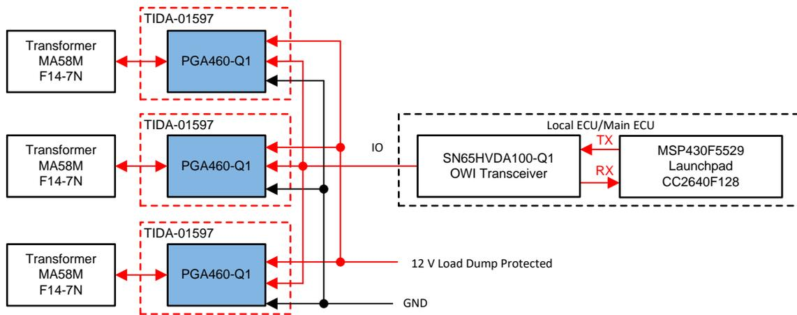
Figure 1. TIDA-01597 Block Diagram
