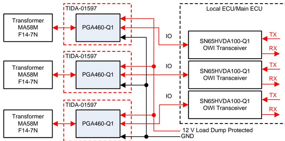
Figure 11. TCI System Architecture
