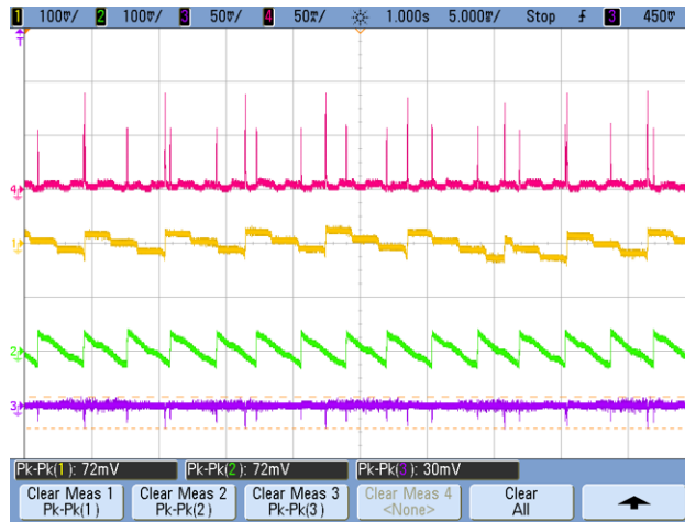
Figure 46. Pink Waveform Shows 100-ms Advertising Time for BLE
