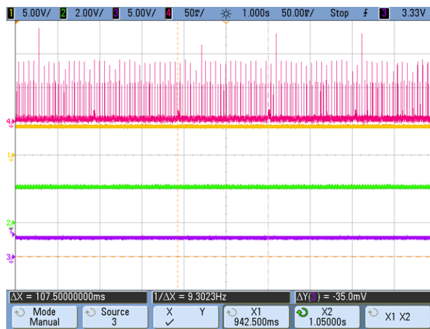
Figure 46. Pink Waveform Shows 100-ms Advertising Time for BLE
