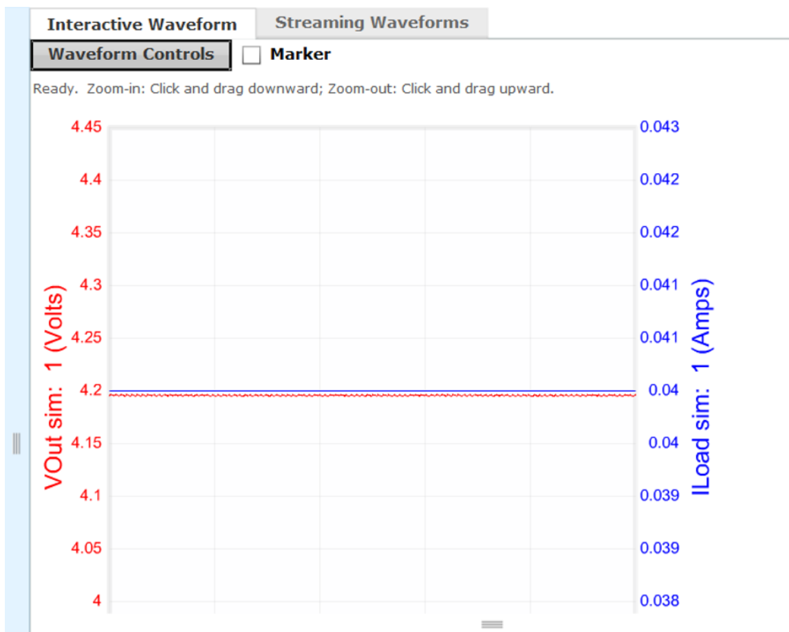
Figure 11. WEBENCH® Simulation for TPS61099 Boost Converter (Test Results)
