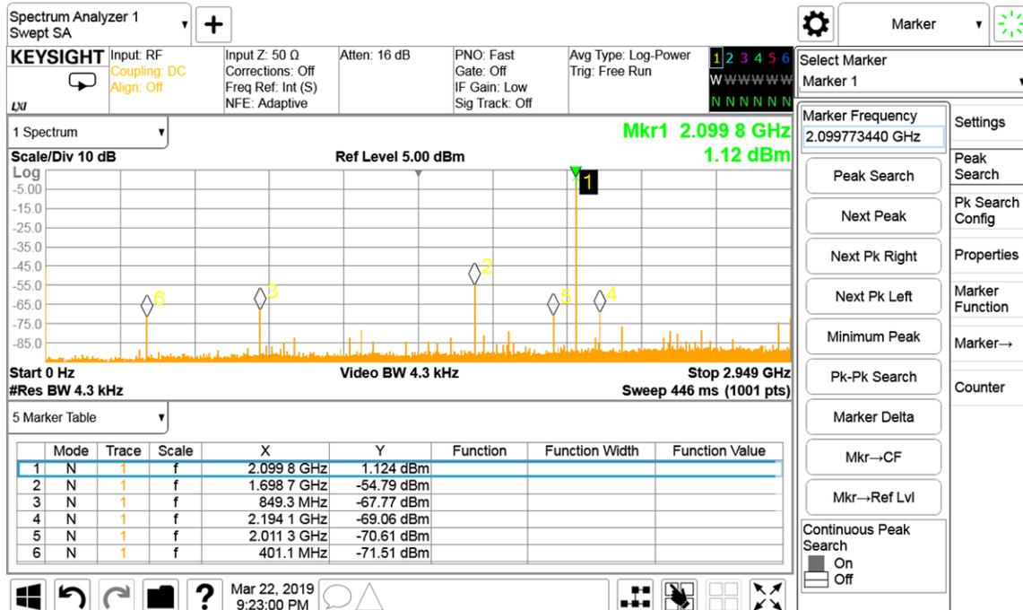
Figure 34. DAC Spectrum at 2100-MHz Output ( $\pm 250$  MHz)
