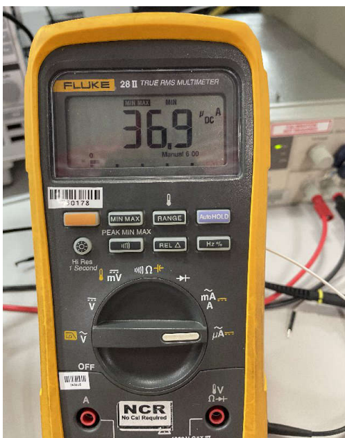
Figure 4-5. System I_Q Without an MCU
