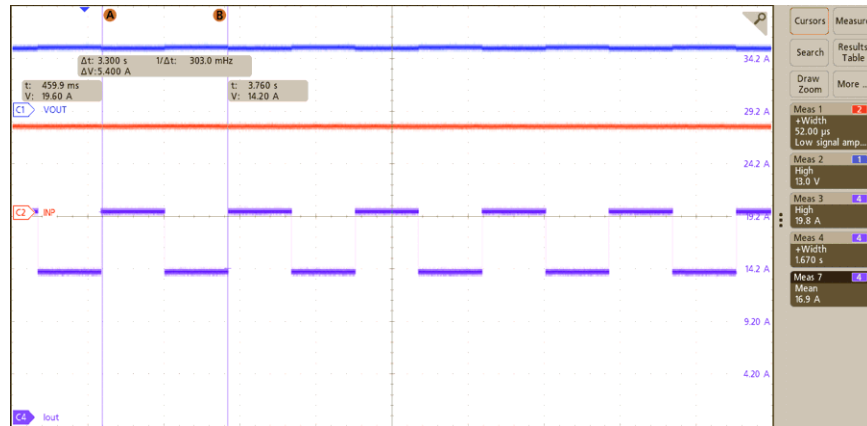
Figure 4-13. PWM Overcurrent Test
