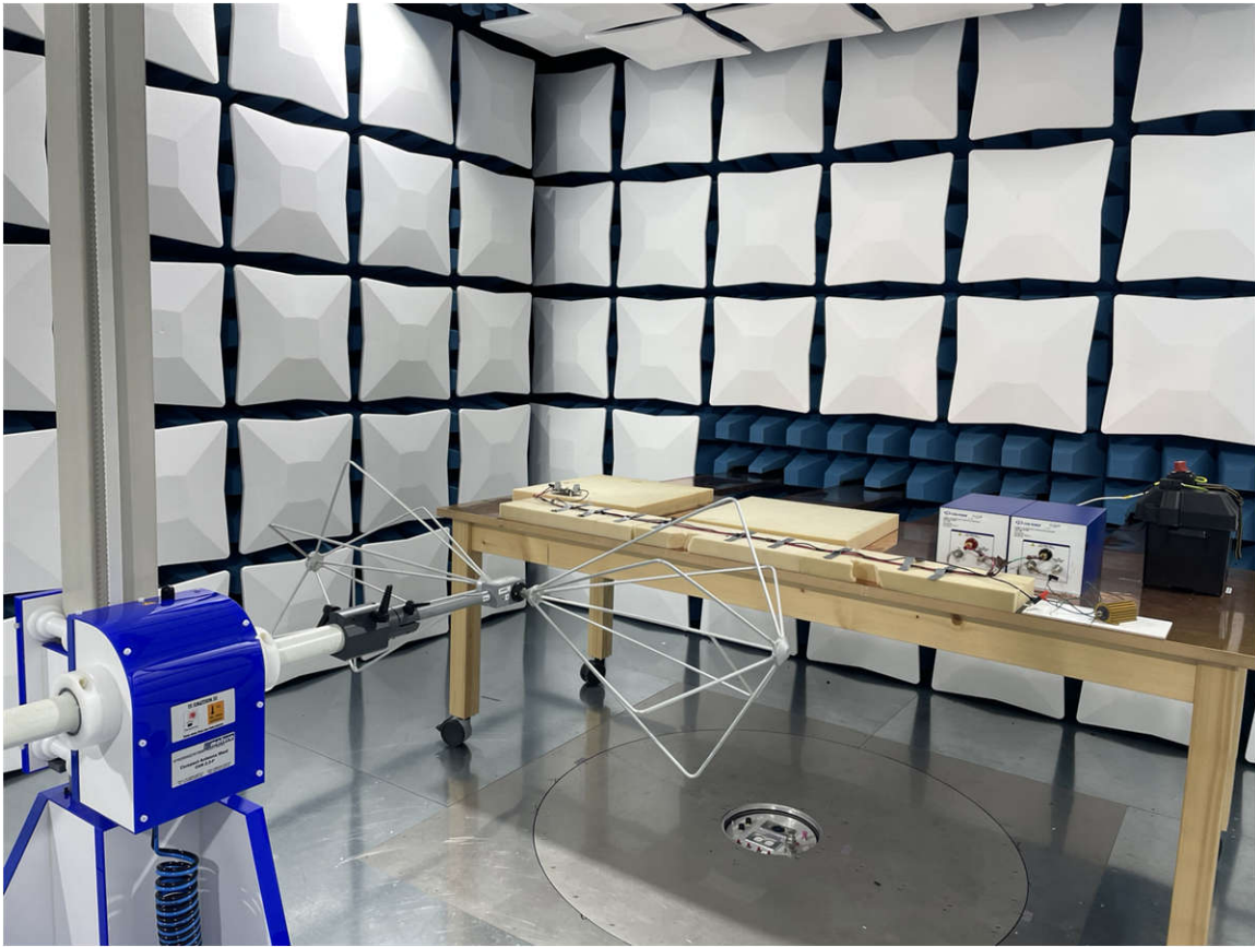
Figure 4-26. RE Setup With a Biconical Antenna: 30MHz to 200MHz
