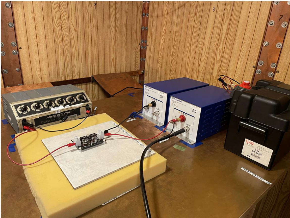
Figure 4-18. Conducted Emissions Test Setup
