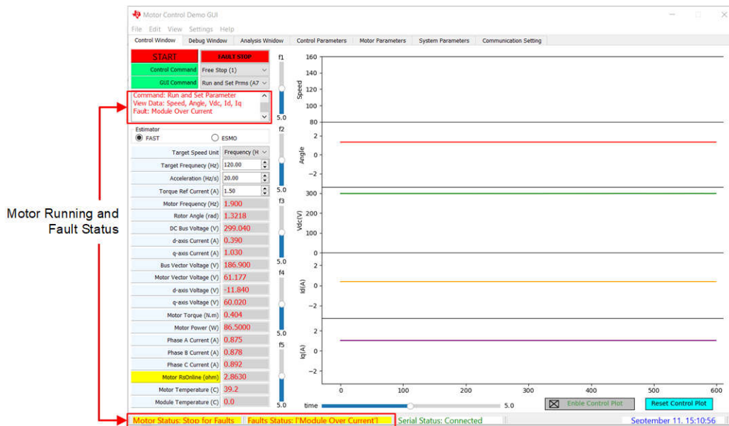
Figure 3-12. Fault Status Monitor
