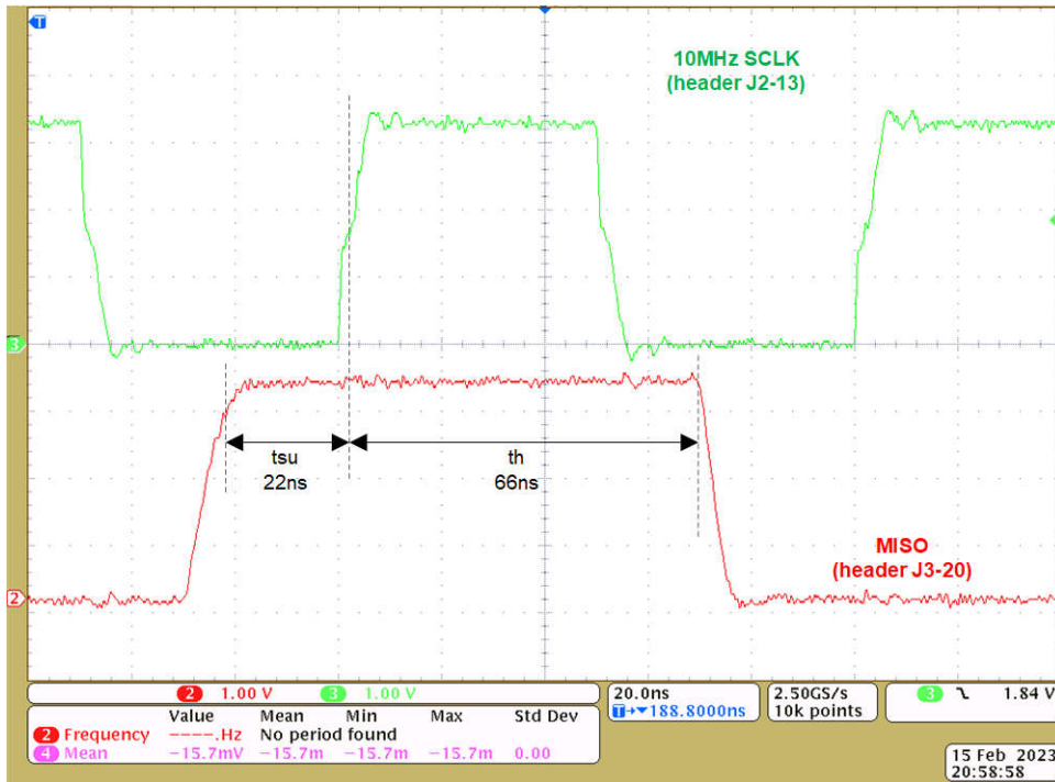
Figure 4-17. MISO and SCLK at MCU Headers J2 and J3
