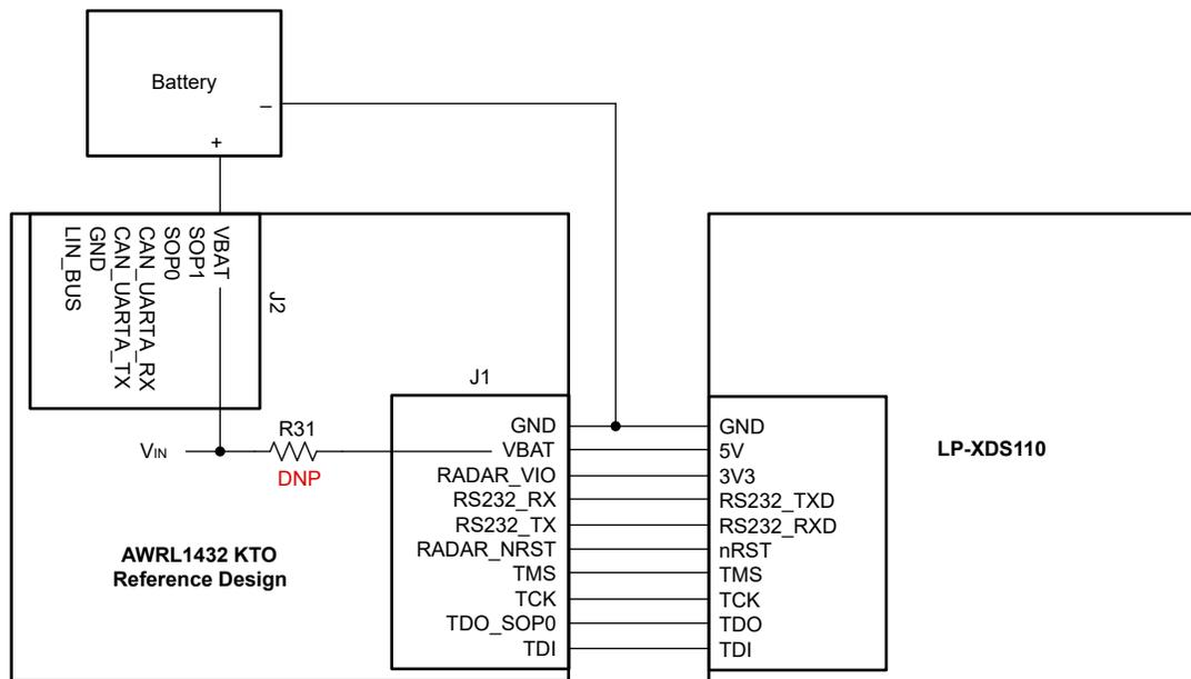
**Figure 3-1. Connections in Primary Power Up Option**
