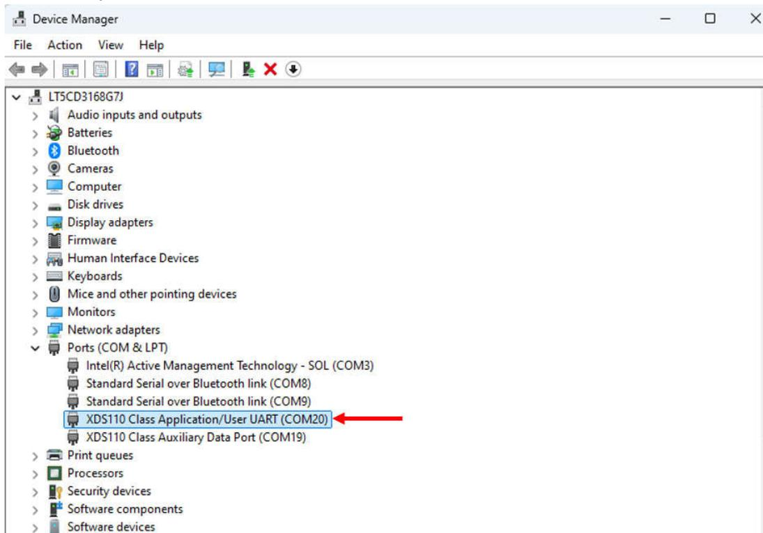
**Figure 3-5. Determine COM Port**
