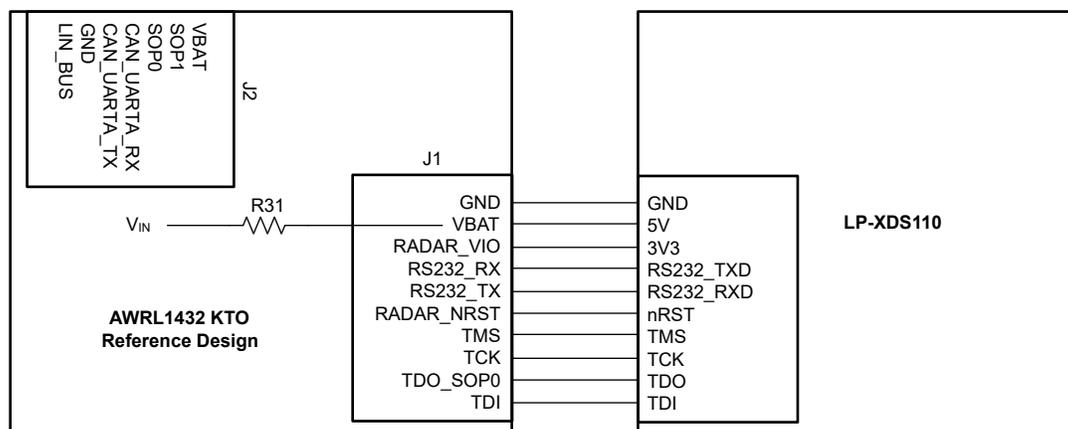
Figure 3-2. Connections in Secondary Power Up Option
