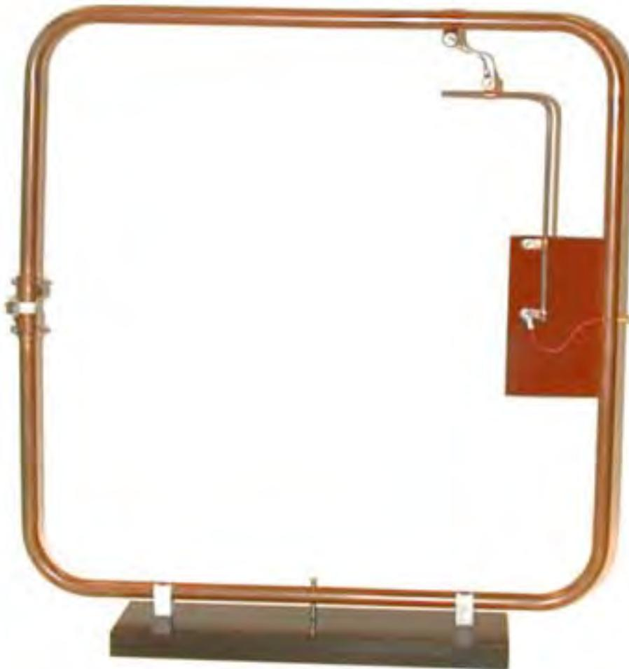
**Figure 14. Gamma Matched Antenna**
