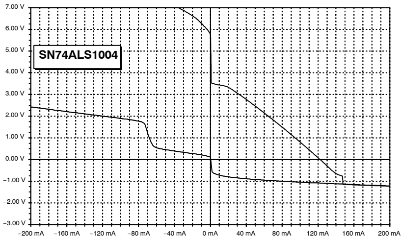
Figure 41. Output Characteristics of the SN74ALS1004
