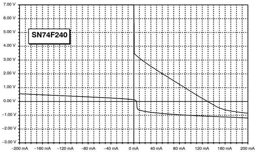
Figure 47. Output Characteristics of the SN74F240
