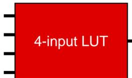
Capable of realizing any combinatorial Boolean equation of up to four inputs.
