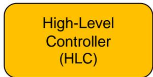
An event-driven block which can handle up to four concurrent events. The event can be an activity on any of the other block outputs. A predefined set of operations is executed when each event occurs. The HLC also provides a data exchange and interrupt mechanism to the CPU subsystem. There are four working registers (R0, R1, R2, and R3) which can be used for basic operations, and to modify or set up values for the three counter blocks.
