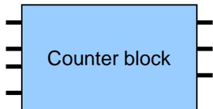
Configurable either as an adder, a counter, or a shifter. As an adder, it can either add or subtract. As a counter, it can count up or count down. As a shifter, it can shift left or right. The counter event inputs, as well as the reset input, may be freely connected to any of the other submodules in the same tile.
