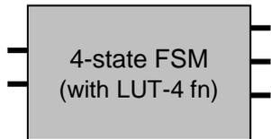
Configurable either as a single four-state finite state machine, or as two independent two-state finite state machines. The FSM accepts two external inputs, and generates two state outputs and one combinational output. When not used as a state machine, the FSM submodule can accept two external inputs and function as a 4-input LUT.
