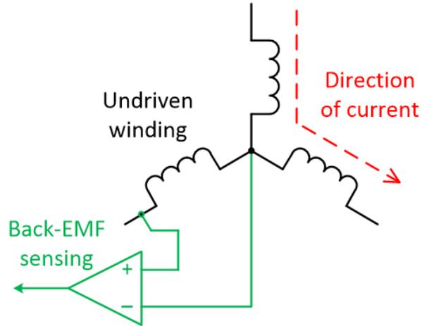
Back-EMF is a sinusoidal or trapezoidal voltage generated on the motor while it is spinning
