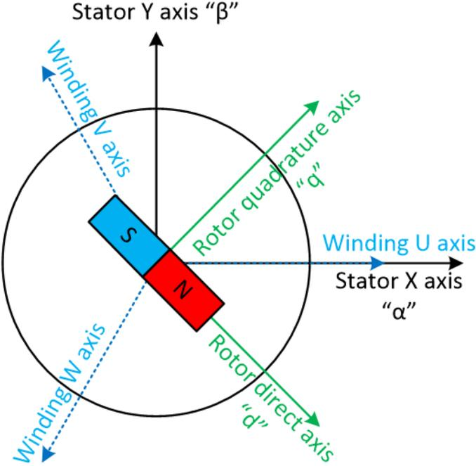
FOC applies all motor torque perpendicular to the rotor
