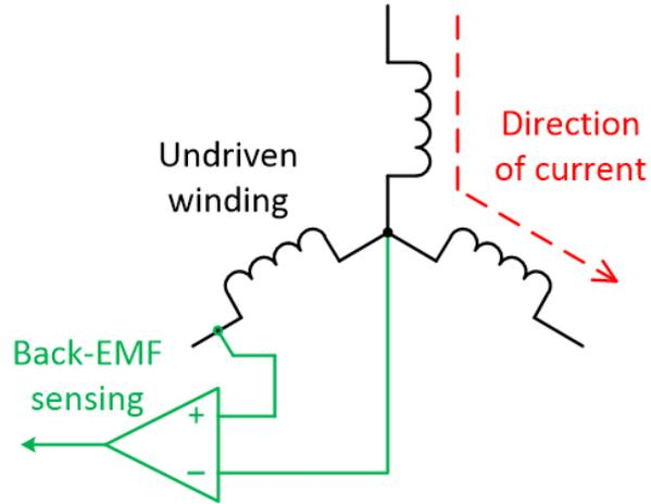
Figure out where the motor is through Back-EMF
