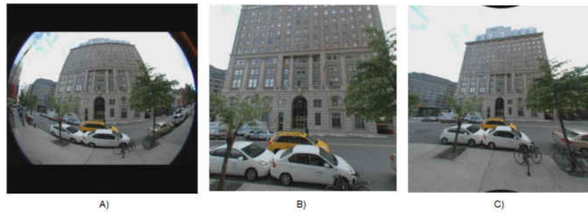
Figure 5-1. Lens Distortion Correction: A) The unprocessed frame from a fisheye lens, B) Front perspective output image C) Intermediate mesh image - warp and interpolate to project image into full-resolution rectangular format using equisolid fisheye projection model
