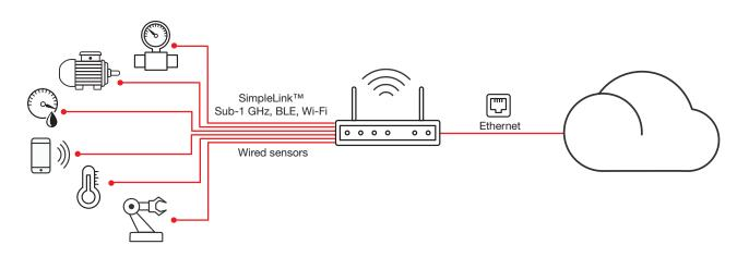
Figure 3. SimpleLink MSP432E4 MCUs are the industry's most integrated Arm<sup>®</sup> Cortex<sup>®</sup>-M4 MCUs, with an integrated 10/100 media access controller plus physical layer (MAC+PHY) for implementing intelligent gateways.
