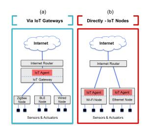
Figure 2. An IoT gateway can simplify connectivity design for sensor nodes by centralizing IoT functionality in the gateway. Nodes connect to the IoT via a gateway using both wired and wireless technology (a); nodes connect directly to the internet using a WAN connection such as Wi-Fi or Ethernet (b).
