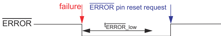
Figure 22-19. \overline{\text{ERROR}} Pin Timing - Example 3
