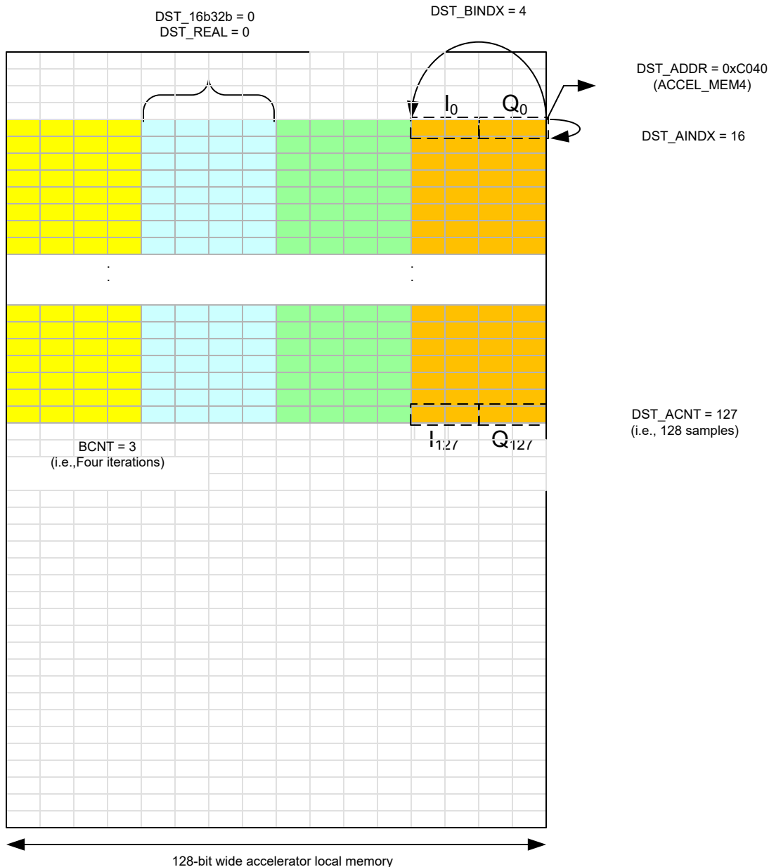
Figure 10-10. Output Formatter Destination Memory Access Pattern (Example)
