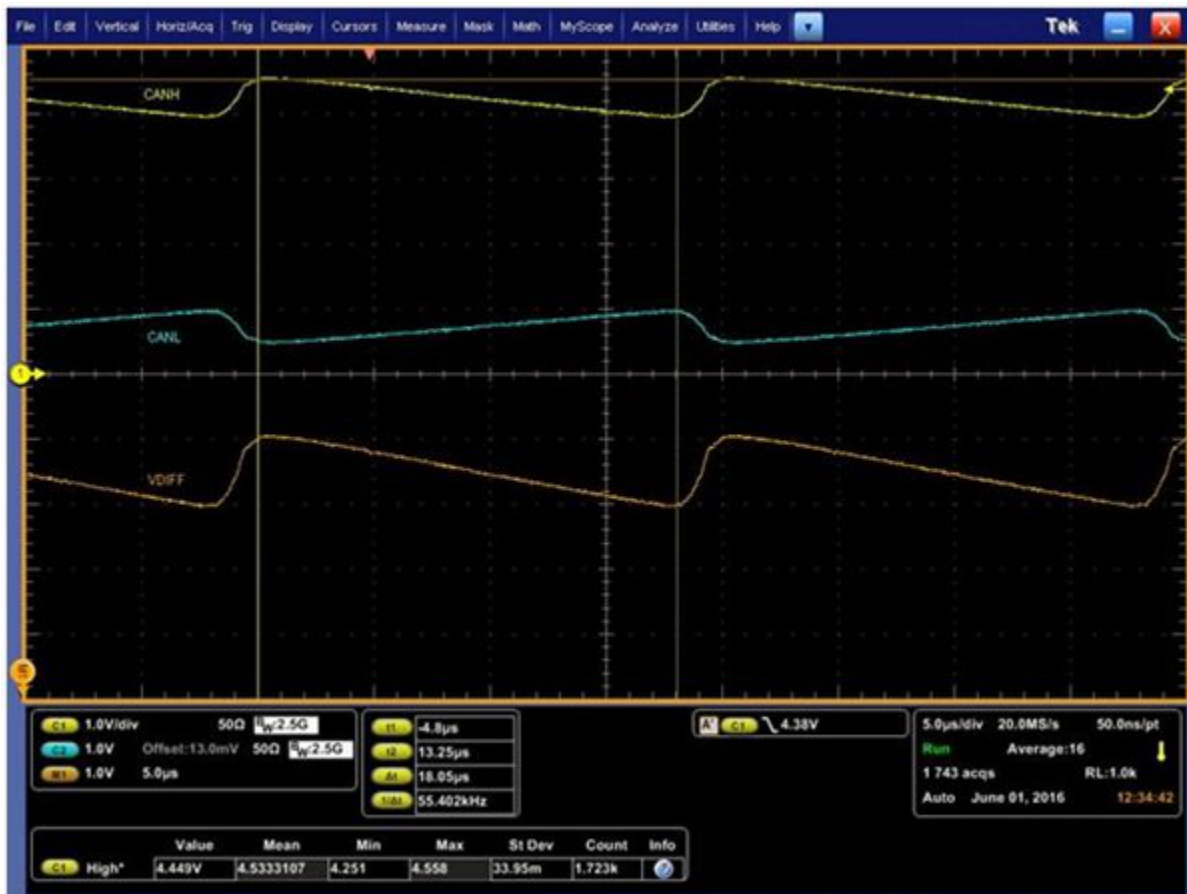
Figure 4. CAN Bus Signals with No Termination (Both Missing)
