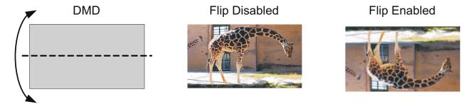
Figure 2-2. Image Short-Axis Flip Example
