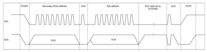
Figure 1-1. I<sup>2</sup>C Read Command Waveform Diagram
