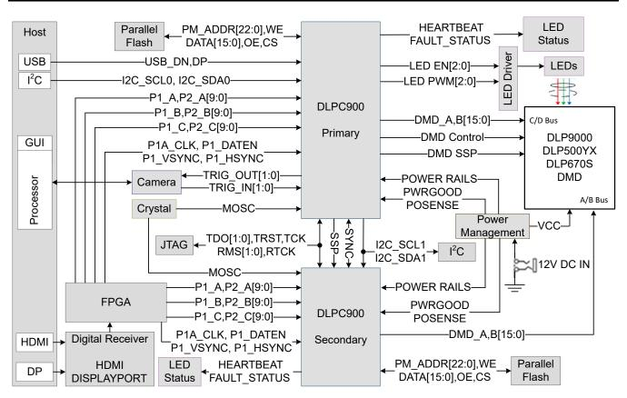
Figure 2-5. DLPC900 Dual Controller System Block Diagram
