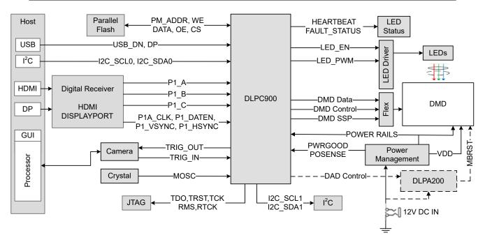
Figure 2-4. DLPC900 Single Controller System Block Diagram
