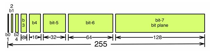
Figure 2-7. Bit Partition in a Frame for an 8-Bit Monochrome Image
