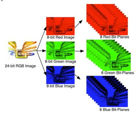
Figure 2-6. Bit-Planes of a 24-Bit RGB Image
