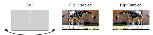
Figure 2-1. Image Long-Axis Flip Example
