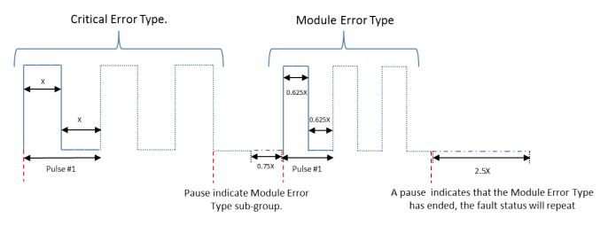
Figure 3-1. DLPC900 FAULT\_STATUS Format
