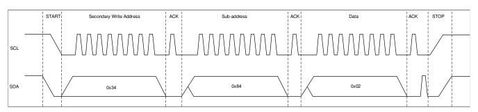
Figure 1-3. I<sup>2</sup>C Write Command Waveform Diagram
