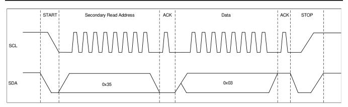
Figure 1-2. I<sup>2</sup>C Read Data Waveform Diagram
