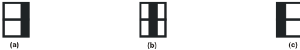
Figure 11. Clock selection jumper configurations: (a) Transformer (default); (b) Single-ended clock; (c) Future CLK input option based on U1. Both (b) and (c) configurations need some modifications on the PCB.
