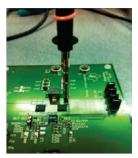
Figure 10. Testing Switch Node
