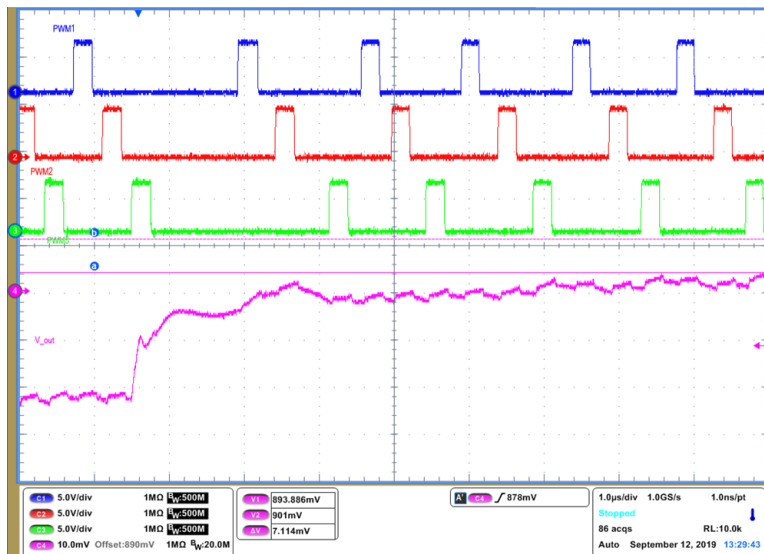
Figure 11. Measurement of Margin at the Upper Limit of Output Voltage
