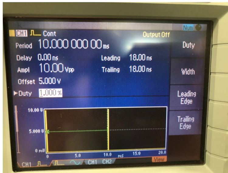
Figure 37. Arbitrary Waveform Generator Setup for Modulating Gate of Power FET
