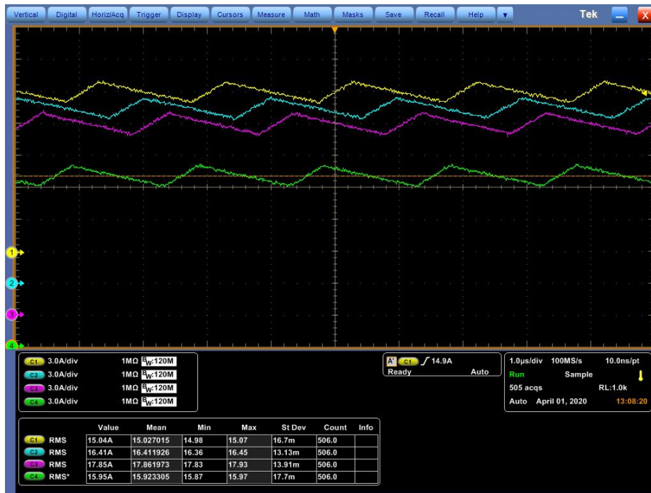
Figure 18. Current Sharing 65Amps Total eLoad Current
