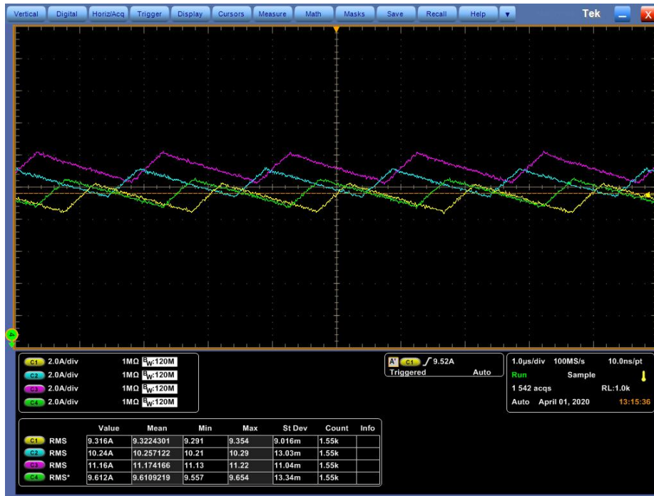
Figure 17. Current Sharing 40Amps Total eLoad Current
