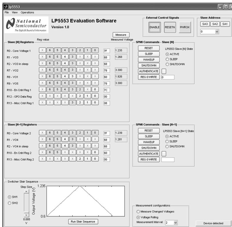
Figure 4. LP5553 Evaluation Software (Button View)
