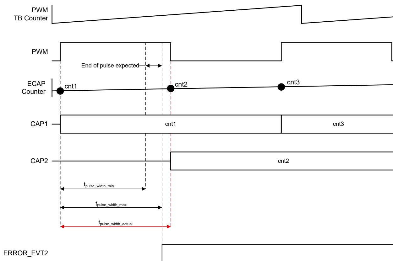
Figure 21-12. ECAP Signal Monitoring Unit Pulse Width Error Example
