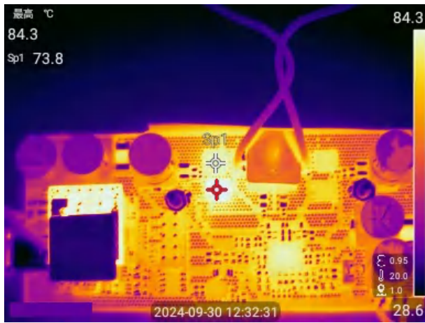
Figure 2-9. OTG mode, 42V Battery 10S to 48V 5A
