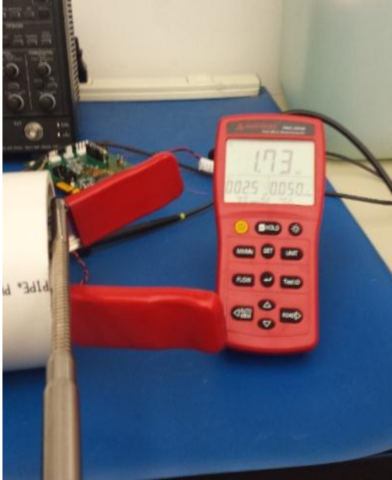
Image showing the use of the anemometer to measure air flow speeds.
