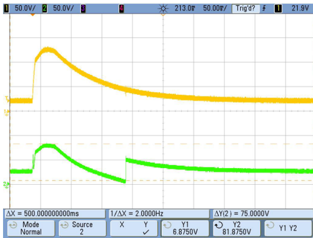
Figure 46. TIDA-01167 Unsuppressed Load Dump Behavior for 24 V
