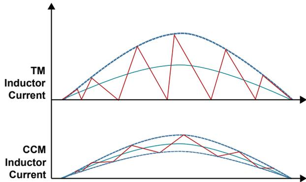
Figure 27 – CrCM/TM and CCM inductor ripple current comparison.
