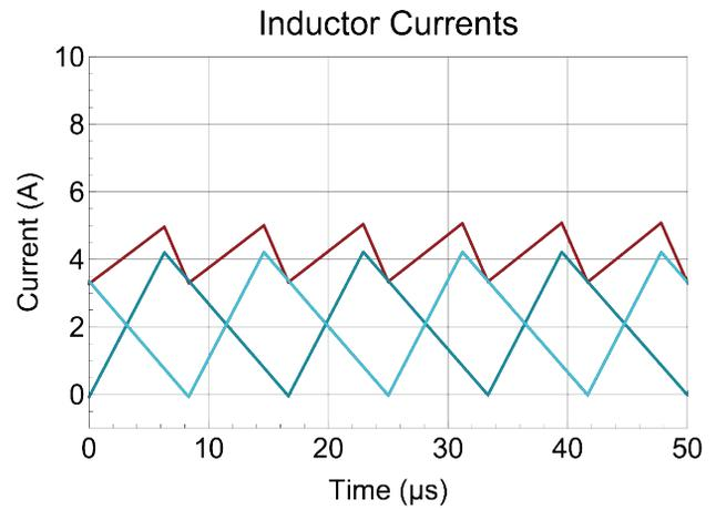
Figure 23 – Interleaved boost inductor currents and total input current ripple.
