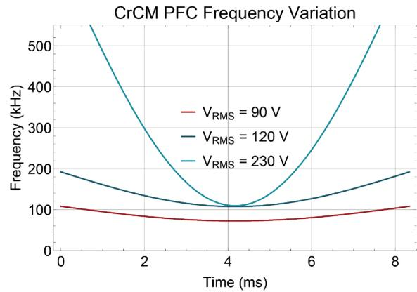
Figure 10 –  $F_{SW}$  variation over 1/2 line cycle.
