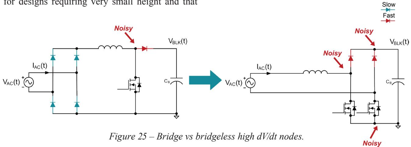
Figure 25 – Bridge vs bridgeless high  $dV/dt$  nodes.
