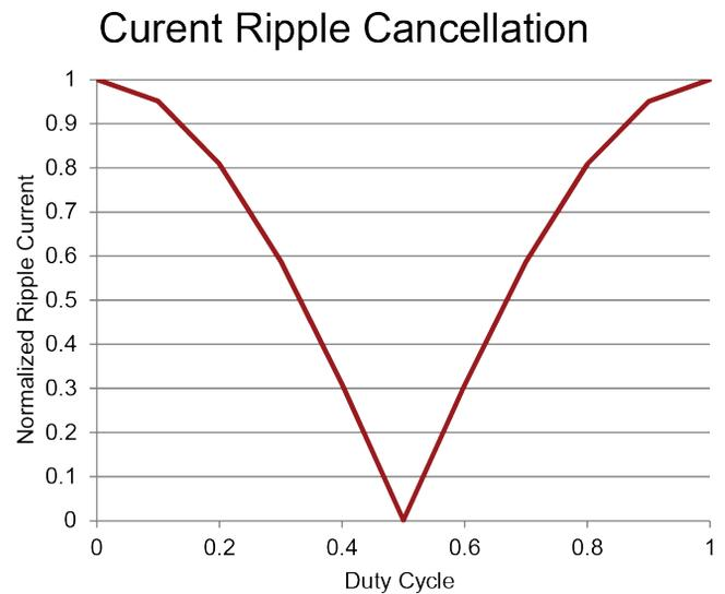
Figure 24 – Ripple current cancellation for two stage interleaved boost.
