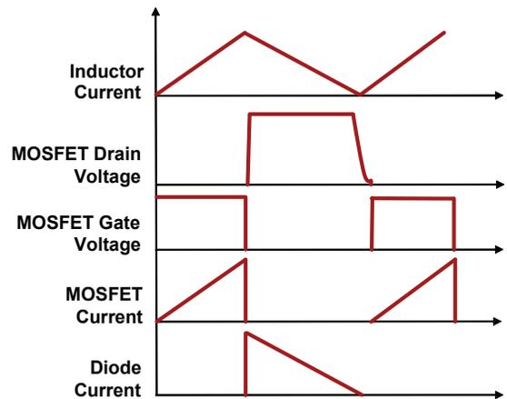
Figure 8 – Boost converter waveforms.
