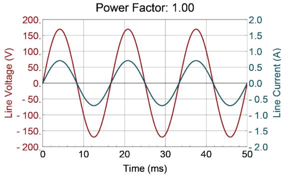
Figure 1 – Input voltage and current for  $PF=1$ .
