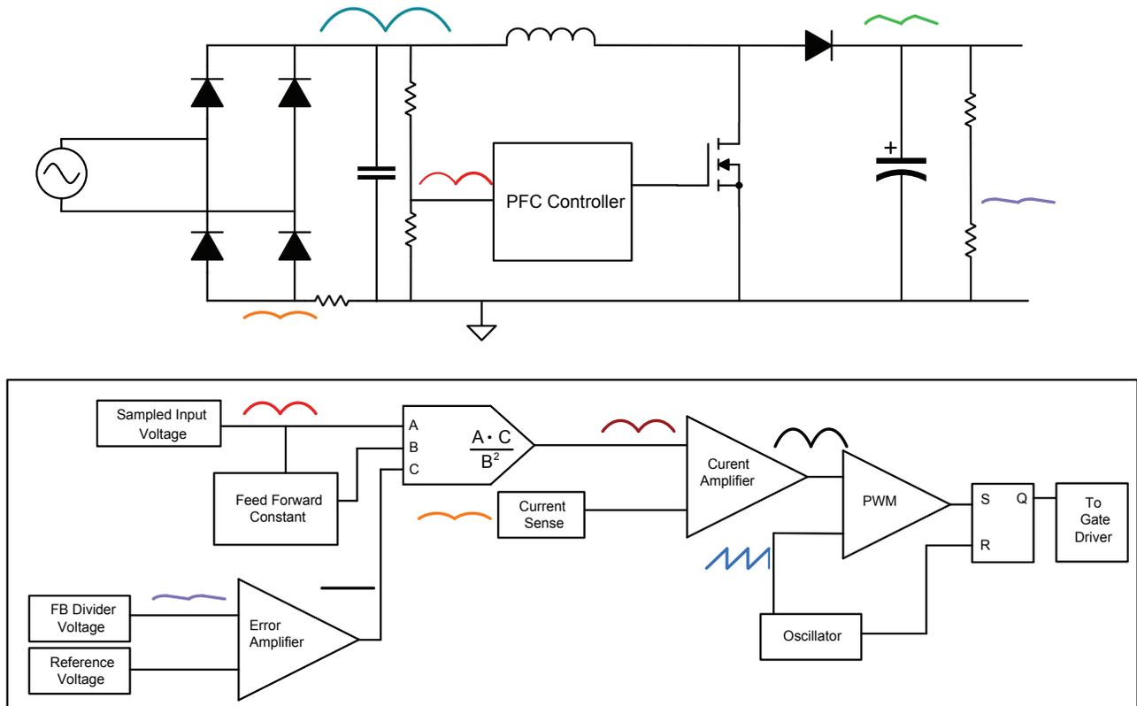
Figure 19 – CCM PFC block diagram using average current mode control.
