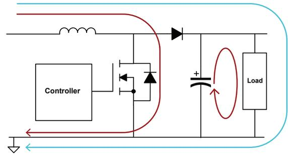
Figure 7 – Boost converter power paths.
