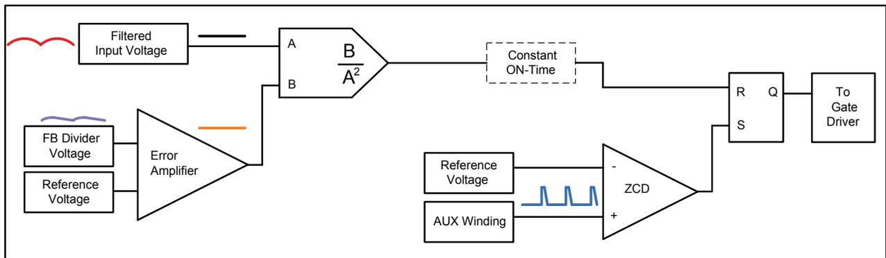
Figure 18 – CrCM PFC block diagram using constant on-time.
