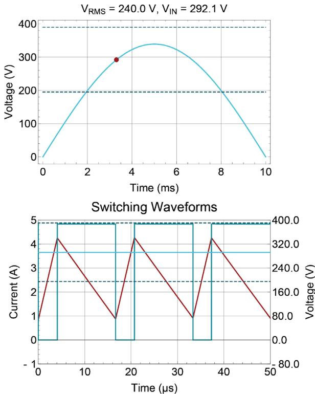
Figure 20 – Inductor current and MOSFET drain waveforms near peak of AC line.
