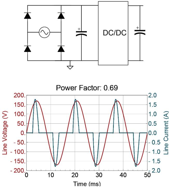
Figure 4 – AC/DC power supply input voltage and current.
