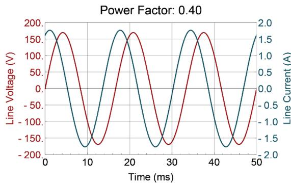
Figure 2 – Input voltage and current with  $PF=0.4$  due to phase delay.
