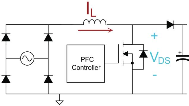
Figure 11 – Simplified boost PFC schematic.
