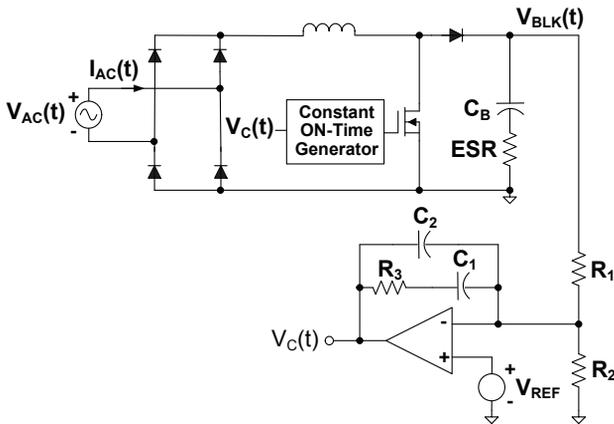
Figure 16 – PFC behavioral model and compensation.
