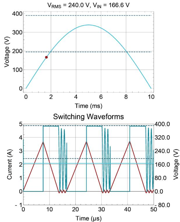
Figure 21 – Inductor current and MOSFET drain waveforms near AC zero crossing.
