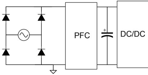
Figure 6 – Introduction of power factor correction stage.
