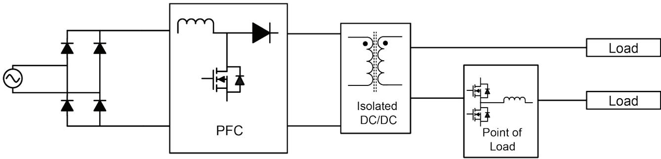
Figure 9 – AC/DC power supply block diagram.
