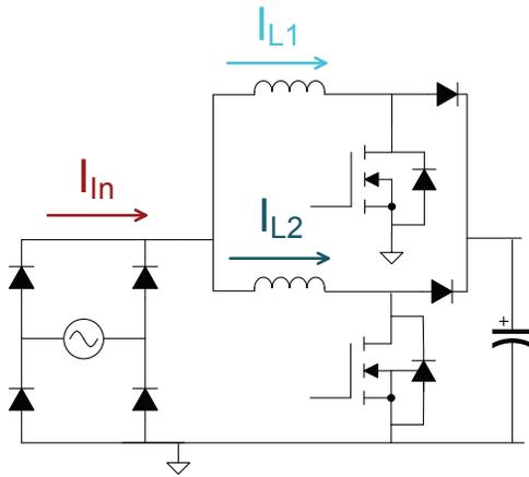
Figure 22 – Interleaved boost PFC.
