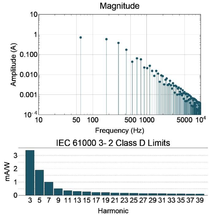
Figure 5 – Input current harmonic content and IEC61000-3-2 Class D limits.
