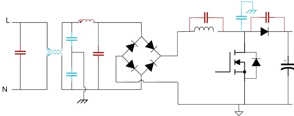
Figure 29 – Boost parasitics and EMI filtering.
