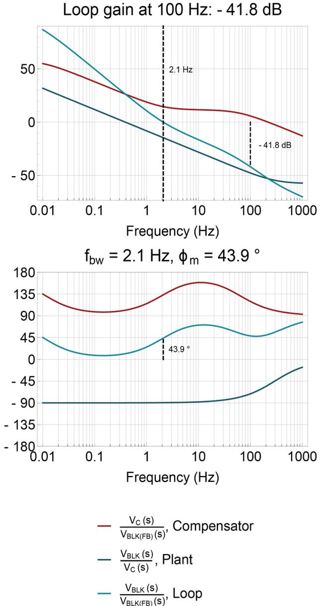
Figure 17 – PFC plant, compensator and closed loop gain and phase.
