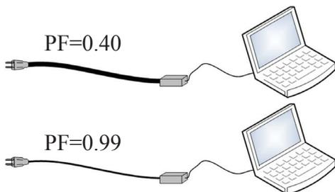
Figure 3 – Laptop cable comparison.
