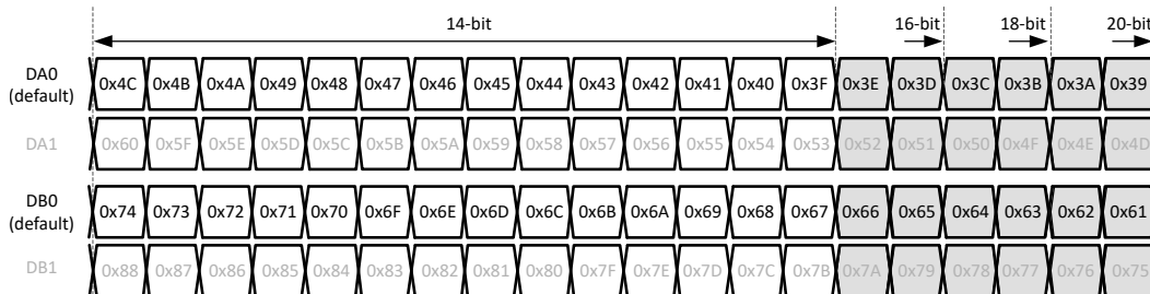
Figure 7-42. 1-wire output bit mapping
