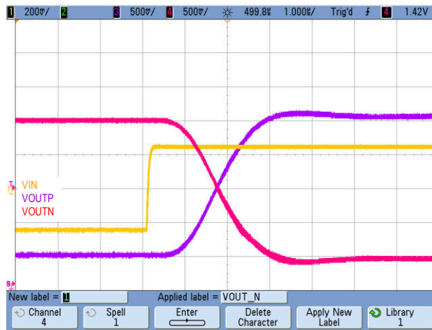
Figure 8-4. Step Response of the AMC1301
