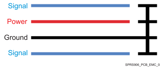
Figure 7-13. Guard Ring Routing
