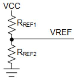
**Figure 7-3. Resistor divider connected to the VREF pins**
