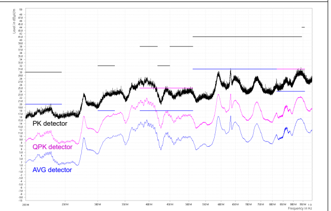
Figure 8-20. CISPR 25 Class 5 Radiated EMI, Log Antenna, Vertical Polarization, 200MHz to 1GHz
