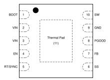
Figure 4-2. DPR Package 10-Pin (WSON) Top View
