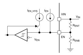
Figure 6-3. System UVLO By Enable Dividers
