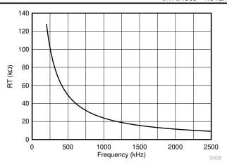
Figure 6-4. R<sub>T</sub> vs Frequency Curve
