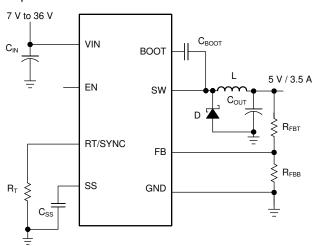
Figure 7-1. Application Circuit, 5V Output
