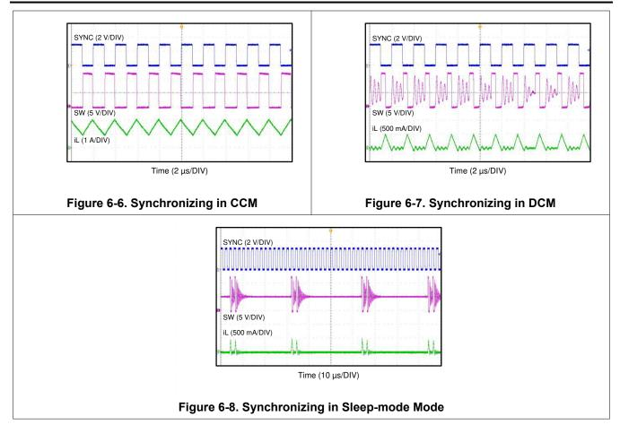
For spread spectrum option, the internal frequency dithering is diabled if the device is synchronized to an external clock.
