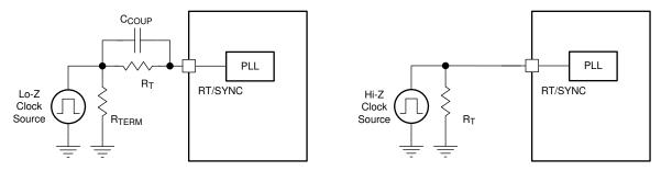
Figure 6-5. Synchronizing to an External Clock
