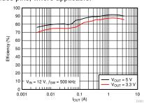
**Efficiency vs Output Current**
