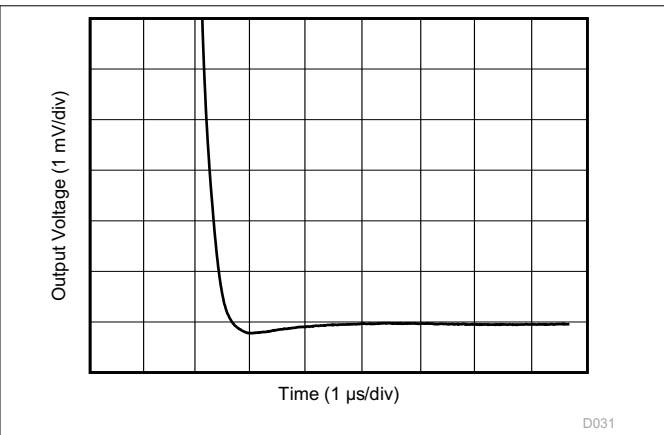
Figure 5-26. Large-Signal Settling Time (Negative)
