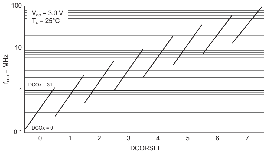
Figure 5-10. Typical DCO Frequency
