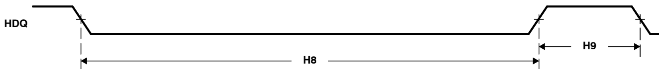
Figure 5-39. HDQ/1-Wire Break (Reset) Timing
