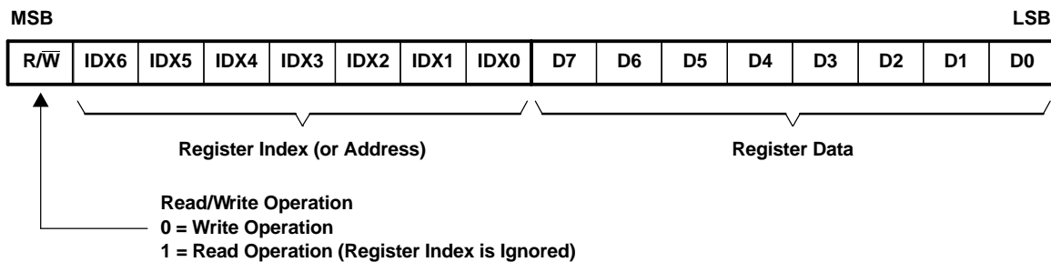
Figure 24. Control Data Word Format for MDI
