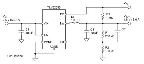
Figure 4. 1.8-V Output Voltage Application
