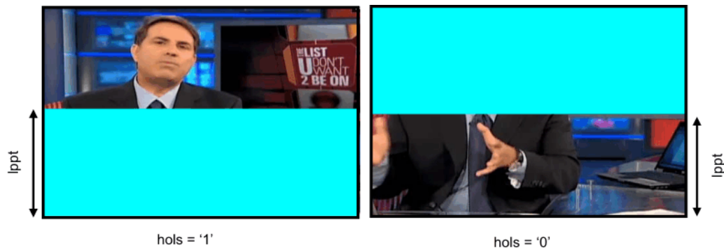
Figure 25-15. Subpicture Output with HOLS Bit Variations
