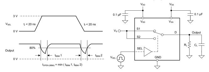
Figure 6-6. Break-Before-Make Delay Measurement Setup
