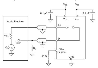
Figure 6-13. THD + N Measurement Setup
