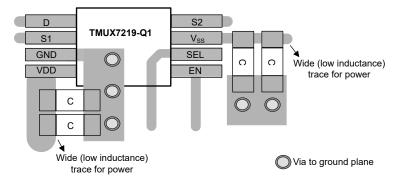
Figure 8-3. TMUX7219-Q1DGK Layout Example
