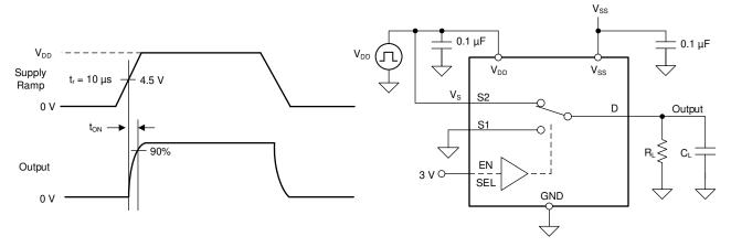
Figure 6-7. t<sub>ON (VDD)</sub> Time Measurement Setup
