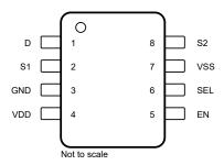
Figure 4-1. DGK Package, 8-Pin VSSOP (Top View)
