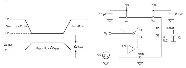
Figure 6-9. Charge-Injection Measurement Setup
