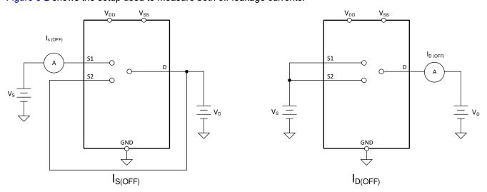
Figure 6-2. Off-Leakage Measurement Setup
