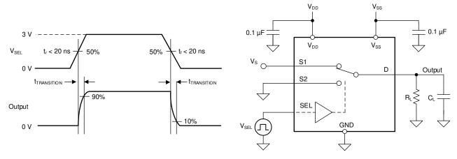
Figure 6-4. Transition-Time Measurement Setup
