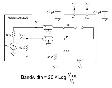
Figure 6-12. Bandwidth Measurement Setup
