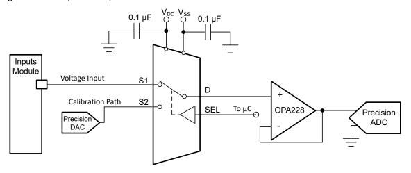
Figure 8-1. Calibration Path Switching for Data Acquisition
