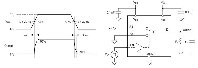
Figure 6-5. Turn-On and Turn-Off Time Measurement Setup
