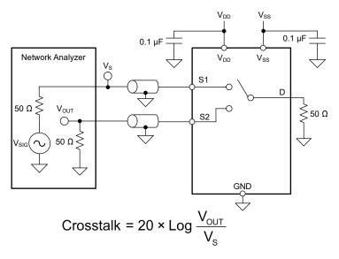
Figure 6-11. Crosstalk Measurement Setup
