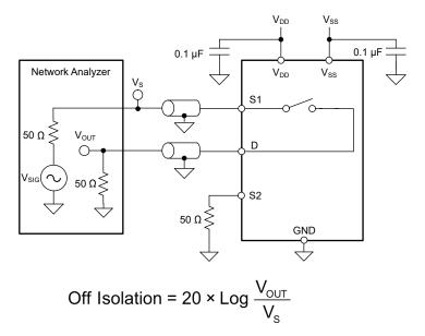
Figure 6-10. Off Isolation Measurement Setup
