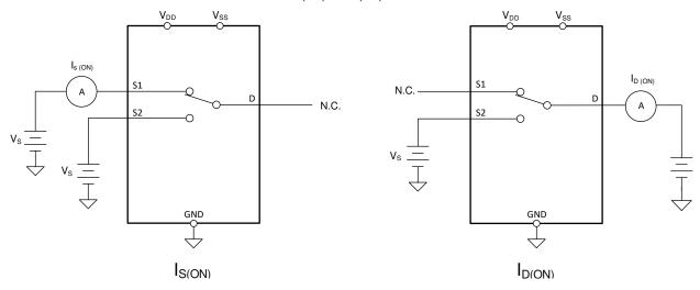
Figure 6-3. On-Leakage Measurement Setup
