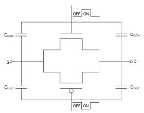
Figure 7-1. Transmission Gate Topology
