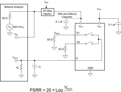
$PSRR = 20 \times Log \frac{V_{OUT}}{V_{IN}}$
