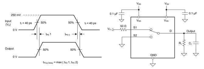
Figure 6-8. Propagation Delay Measurement Setup
