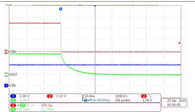
Figure 7-26. Turn-Off at 3.6 V (Open Load)
