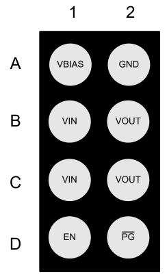
Figure 4-1. TPS22999 YCH Package, 8-Pin DSBGA (Top View)
