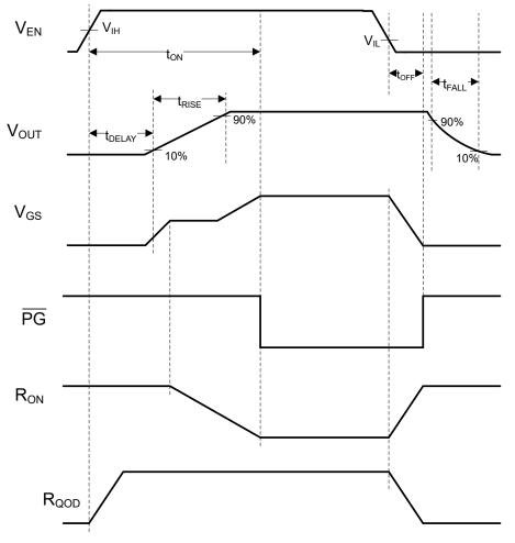
Figure 5-1. TPS22999 Timing Diagram
