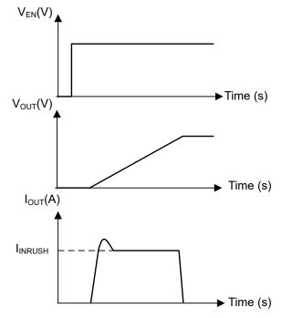
Figure 6-1. Regulated Inrush Current Behavior
