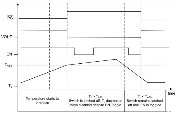
Figure 6-2. Thermal Shutdown Behavior
