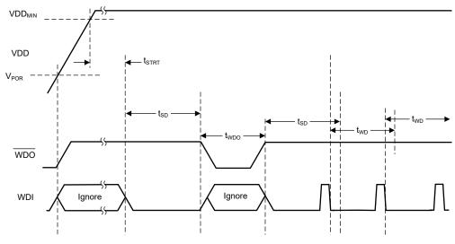
Figure 7-8. t<sub>SD</sub> Frame Behavior
